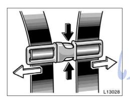
4. Compress the shoulder belt clip to separate the right and left shoulder belts.
