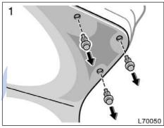
Use a flat-bladed screwdriver. Remove and install the cover clips as shown in the following illustrations. تلفن شبانه روزی:
