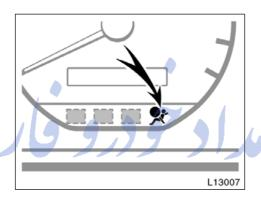
This indicator comes on when the ignition key is turned to the "ACC" or "ON" position. It goes off after about 6 seconds. This means the SRS side airbags are operating properly.
