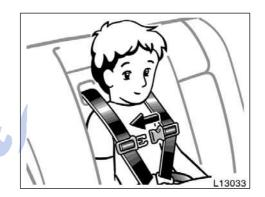
Sit the child on the child seat. Place a shoulder belt over each shoulder. Insert the tabs into the buckle.
