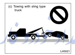
(c) Towing with sling type truck
