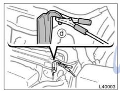
Connecting point for 5S-FE engine
