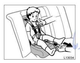
Pull the seat belt adjustment strap (gray tab) firmly until the shoulder belts are snugly adjusted around the child's shoulders.
