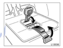
11. To store the built-in child restraint, fasten the shoulder belt clip and return the seat belt buckle using the fastener tapes. Fold up the seat belt adjustment strap (gray tab) in the seat so that the edge of the strap does not come out the raised child restraint seat cushion. Raise the child restratraint seat cushion and reinstall the head restraint and upper pad correctly by inserting the posts into the holes.
