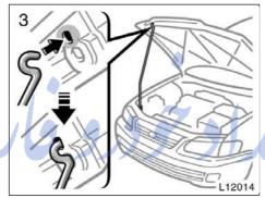
3. Hold the hood open by inserting the support rod into the slot.
