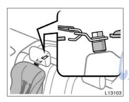
To comply with Canadian Motor Vehicle Safety Standards, this model sold in Canada is provided with a bracket set in the glovebox, designed for use with any of the 3 anchor locations shown in the illustration.
