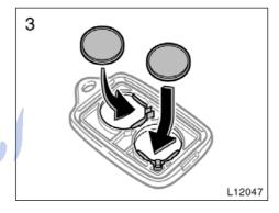
3. Put new transmitter batteries with negative (-) side up.
