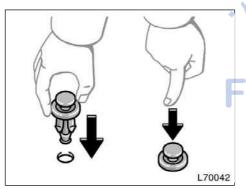
Installing the cover clips
