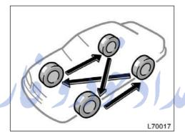
To equalize the wear and help extend tire life, Toyota recommends that you rotate your tires approximately every 12000 km (7500 miles). However, the most appropriate timing for tire rotation may vary according to your driving habits and road surface conditions.
