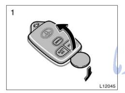
1. Using a coin or equivalent, open the transmitter case.
