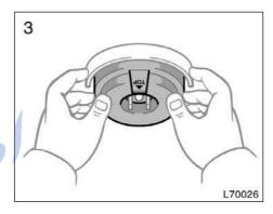
Install the rubber cover with the "TOP" mark upward, and snuggle on the boss. Insert the connector. Then install the plastic cover.
