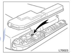
If the headlights or other electrical components do not work, check the fuses. If any of the fuses are blown, they must be replaced.
