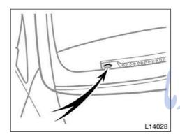
The daytime running light control sensor is on the top of the passenger's side instrument panel.
