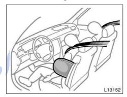
The SRS (Supplemental Restraint System) side airbags are designed to provide further protection for the driver and front passenger when added to the primary protection provided by the seat belts.
