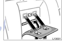
6. Press the removable pad against the fastener tapes and install the pad to the seatback. Make sure the belts go through the slots in the pad.
