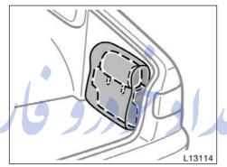
Insert the head restraint and upper pad into the storage bag. Then place the storage bag into the trunk by attaching with Velcro.
