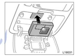
Remove the paper strip covering the adhesive on back side of loop and adhere loop to back side of the transmitter near center.
