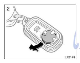
2. Remove the discharged transmitter battery.
