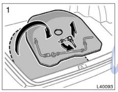
1. Remove and turn over the spare tire cover. Remove the front towing eyelet by turning it as shown in the illustrations.
