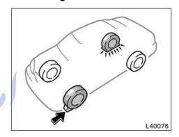
When blocking the wheel, place a wheel block from the front for the front wheels or from the rear for the rear wheels.
