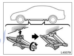
Position the jack at the correct jack point as shown. Rotate the load rest
