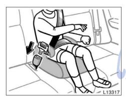
Sit the child on a booster seat. Run the lap and shoulder belt through or around the booster seat and child following the instructions provided by its manufacturer and insert the tab into the buckle taking care not to twist the belt.
