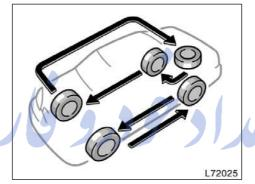
With a spare tire of the same wheel type as the installed tires
