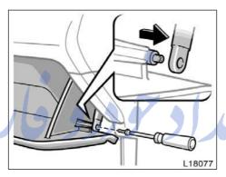
Open the glove box. Remove the 2. screw with a Phillips-head screw-driver and slide the hook as shown.
