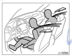
The driver and front passenger's seat belt pretensioners are designed to be activated in response to a severe frontal impact.
