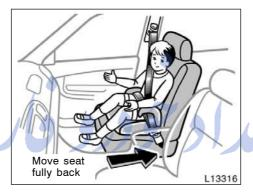
On vehicles with side airbags and curtain shield airbags, do not allow the child to lean against the door or around the door even if the child is seated in the child restraint system. It is dangerous if the side airbag and curtain shield airbag inflate, and the impact could cause death or serious injury to the child.
