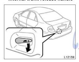
If a person is locked in the trunk, pull down the phosphorescent handle (illuminated for a while) on the inside of trunk lid in case of emergency to open the trunk lid.
