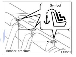
Use the anchor bracket on the package tray behind the rear seat to attach the top strap.
