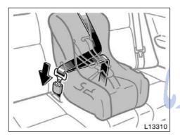
Run the lap and shoulder belt through or around the convertible seat following the instructions provided by its manufacturer and insert the tab into the buckle taking care not to twist the belt. Keep the lap portion of the belt tight.
