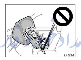
Never install a rear-facing child restraint system on the front passenger seat because the force of the rapid inflation of the front passenger airbag can cause death or serious injury to the child.
