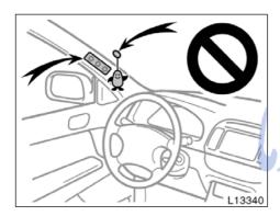
• Do not attach a microphone or any other device or object around the part where the curtain shield airbag activates such as on the windshield glass, side door glass, front and rear pillars, roof side and assist grips. When the curtain shield airbag inflates, the microphone or other device or object will be hurled with great force or the curtain shield airbag may not activate correctly, resulting in death or serious injury.
