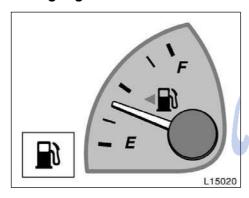
The gauge indicates the approximate quantity of the fuel remaining in the tank when the ignition switch is on.
