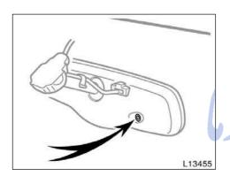
An anti-glare mirror sensor is located on the back side of the mirror. In order not to disturb correct functioning of the mirror, do not touch or cover the sensor with your finger or a piece of cloth, etc.
