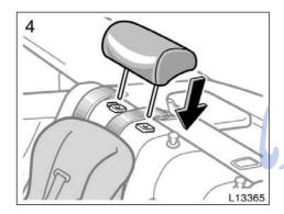
4. Outside anchor brackets only— Replace the head restraint.
