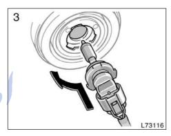
3. Plug in a new bulb into the connector and install it into the mounting
