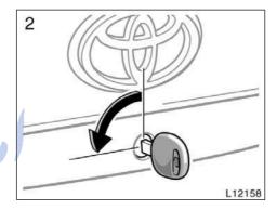
2. Close the trunk lid. Insert the master key and turn it counterclockwise to deactivate the trunk lid lock release lever.
