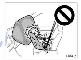
• Never install a rear-facing child restraint system on the front passenger seat even if the "AIRBAG OFF" indicator light is illuminated. In the event of an accident, the impact of the rapid inflation of the front passenger airbag could cause death or serious injury to the child if the rear-facing child restraint system is installed on the front passenger seat.
