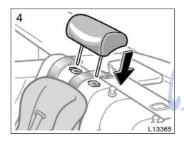
4. Replace the head restraint and lift it up to the uppermost lock position.
