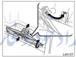
To store the jack, align the hole of the jack head with the vehicle hook. Turn the jack joint until the jack base fits securely with the vehicle body.
