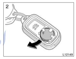
2. Remove the discharged transmitter battery.
