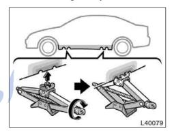
5. Position the jack at the correct jack point as shown. Rotate the load rest 90° from storage position to lifting position.
