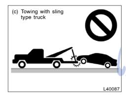
(c) Towing with sling type truck
