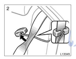
Pinch the two edges of the shoulder belt for the rear seat outside position with your fingers and slide the belt past the slot of the guide as shown above. At this time, the elastic cord must be behind the seat belt.
