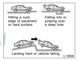
The SRS front airbags may also deploy if a serious impact occurs to the underside of your vehicle. Some examples are shown in the illustration.
