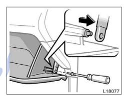
Open the glove box. Remove the screw with a Phillips-head screwi; driver and slide the hook as shown.
