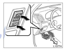
To adjust the position of the accelerator and brake pedals, push the switch.
