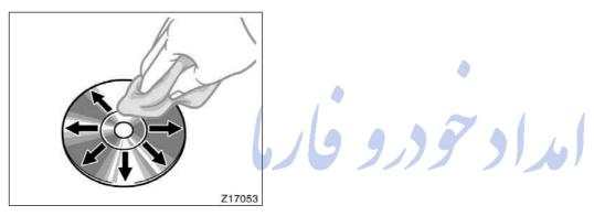
To clean a compact disc: Wipe it with a soft, lint-free cloth that has been dampened with water. Wipe in a straight line from the center to the edge of the disc (not in circles). Dry it with another soft, lint-free cloth. Do not use a conventional record cleaner or anti-static device.
