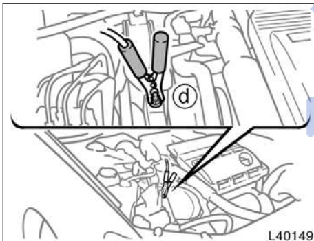
Connecting point for 3.0 L V6 (1MZ-FE) and 3.3 L V6 (3MZ-FE) engines
