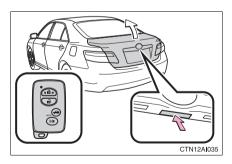
Press the button to unlock the trunk.
