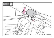
Secure the child restraint using the seat belt lower anchors, and lock the head restraint in place at the lowest position.
