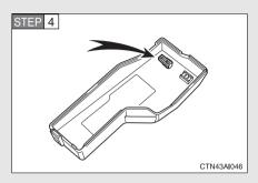
Remove the fuse with the pullout tool.
