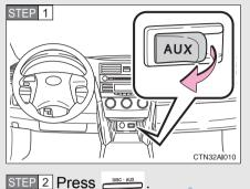
Connect the portable audio device.
