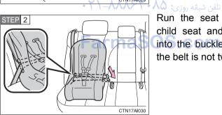
Run the seat belt through the child seat and insert the plate into the buckle. Make sure that the belt is not twisted.
