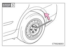
Slightly loosen the wheel nuts (one turn).
