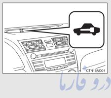
Vehicles with smart key system: The indicator light flashes after the "ENGINE START STOP" switch has been turned OFF to indicate that the system is operating.
