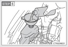
Add engine coolant if necessarv.
