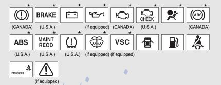
\*: These lights turn on when the "ENGINE START STOP" switch is turned to IGNITION ON mode (vehicles with smart key system) or the engine switch is turned to the "ON" position (vehicles without smart key system) to indicate that a system check is being performed. They will turn off after the engine is started, or after a few seconds. There may be a malfunction in a system if a light does not come on, or if the lights do not turn off. Have the vehicle inspected by your Toyota dealer for details.
