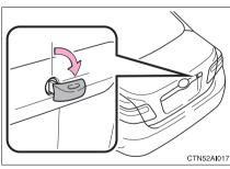
Turn the mechanical key clockwise to open.
