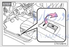
Pull the lever to open the fuel filler door.
