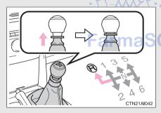
Shift the shift lever to the R position while lifting up the ring section.
