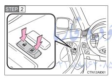
Shift the shift lever to P or N, and press and hold the driver's door ( 😝 or 🔒 ) for lock / switch approximately 5 seconds and then release.
