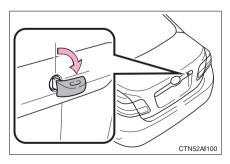
Turn the mechanical key clockwise to open.
