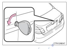
Turn the master key (vehicles without smart key system) or mechanical key (vehicles with smart key system) counterclockwise to lock the trunk opener feature.
