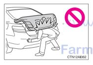
The trunk lid may fall if it is not opened fully. It is more difficult to open or close the trunk lid on an incline than on a level surface, so beware of the trunk lid unexpectedly opening or closing by itself. Make sure that the trunk lid is fully open and secure before using the trunk.
