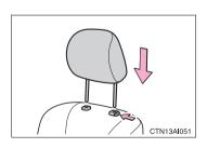
Align the head restraint with the installation holes and push it down to the lock position.
