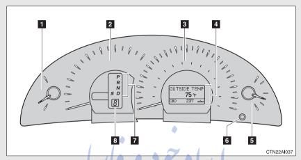
Vehicles with smart key system: The following gauges, meters and displays illuminate when the "ENGINE START STOP" switch is in IGNITION ON mode.
