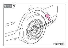
Slightly loosen the wheel nuts (one turn).
