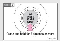
Vehicles with a smart key system: Stop the engine by pressing and holding the "ENGINE START STOP" switch for 3 consecutive seconds or more.
