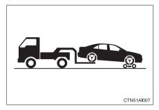
Automatic transmission: Use a towing dolly under the front wheels.
