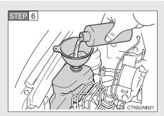
Add engine coolant if necessary.
