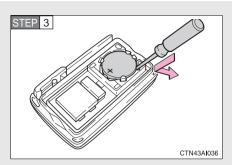
Remove the depleted battery.
