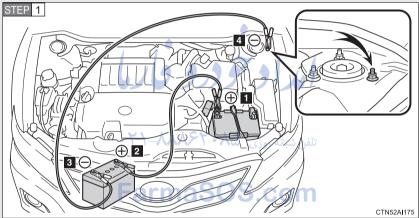
Connecting the jumper cables
