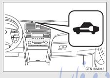
Vehicles with smart key system: The indicator light flashes after the "FNGINE START STOP" switch has been turned OFF to indicate that the system is operating.
