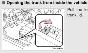
Pull the lever to release the trunk lid.
