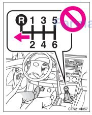
Do not shift the shift lever to R without depressing the clutch pedal.
