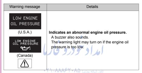
• The following warning indicates the possibility of damage to the vehicle that may lead to an accident. Immediately stop the vehicle in a safe place and allow the engine to cool.
