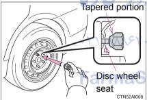
Tighten the nuts until the tapered portion comes into loose contact with the disc wheel seat.
