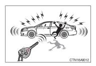
When ((i) is pressed for longer than about one second, an alarm will sound intermittently and the vehicle lights will flash to deter any person from trying to break into or damage your vehicle.
