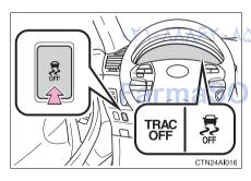
Push and hold the button for more than 3 seconds while the vehicle is stopped to turn off TRAC and VSC.
