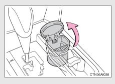
An ashtray can be installed in a cup holder. ( $\rightarrow$ P. 324)
