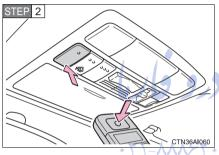
Press and hold down one of the buttons on HomeLink<sup>®</sup> and the button on the transmitter. When the indicator light on HomeLink<sup>®</sup> changes from a slow to a rapid flash after 20 seconds, you can release both buttons.
