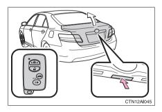
Press the button to unlock the trunk.
