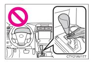
Check that the shift lever is securely set in P. The engine may not start if the shift lever is displaced out of P.
