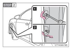
Remove the fender liner clip.
