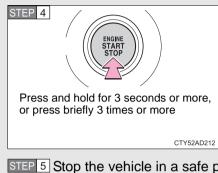
Vehicles with a smart key system: To stop the engine, press and hold the "ENGINE START STOP" switch for 3 consecutive seconds or more, or press it briefly 3 times or more in succession.
