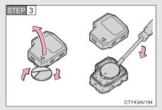
Open the case cover using a coin protected with tape etc. and remove the depleted battery using a small flathead screwdriver.
