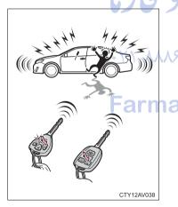
When ((t) is pressed for longer than about one second, an alarm will sound intermittently and the vehicle lights will flash to deter any person from trying to break into or damage your vehicle.
