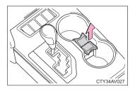
Cup holder insert can be removed.
