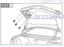
Open the trunk lid and remove the clips. Then partly remove the trunk panel cover.
