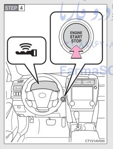
Press the "ENGINE START STOP" switch.
