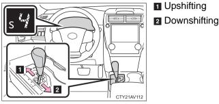
The initial shift range in S mode is set automatically to "5" or "4" according to vehicle speed. However, the initial shift range may be set to "3" if AI-SHIFT has operated while the shift lever was in the D position. ( $\rightarrow$ P. 157)
