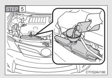
Add engine coolant if necessary.
