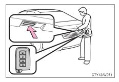
Press the button to unlock the trunk.
