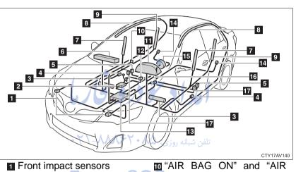
2 Front passenger occupant classification system (ECU and sensors)
