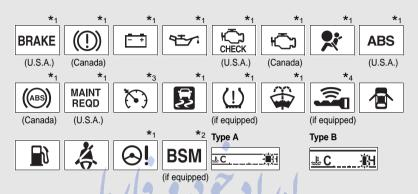
\*1: These lights turn on when the engine switch is turned to the "ON" position (vehicles without a smart key system) or the "ENGINE START STOP" switch is turned to IGNITION ON mode (vehicles with a smart key system) to indicate that a system check is being performed. They will turn off after the engine is started, or after a few seconds. There may be a malfunction in a system if a light does not come on, or if the lights do not turn off. Have the vehicle inspected by your Toyota dealer.
