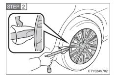
For vehicles with steel wheels, remove the wheel ornament using the wrench.
