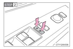
Shift the shift lever to P or N, and press and hold the driver's door lock switch ( $\bigcap$  or  $\bigcap$ ) for approximately 5 seconds and then release.
