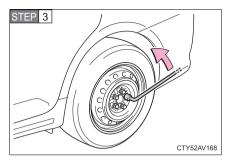
Slightly loosen the wheel nuts (one turn).
