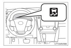
If the vehicle is in danger of slipping or if any of the drive wheels spins, the slip indicator light flashes to indicate that the TRAC/VSC systems are operating.
