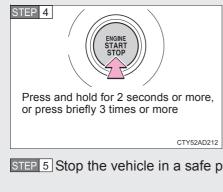
Vehicles with a smart key system: To stop the engine, press and hold the "ENGINE START STOP" switch for 2 consecutive seconds or more, or press it briefly 3 times or more in succession.
