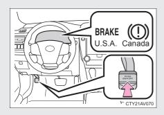
To set the parking brake, fully depress the parking brake pedal with your left foot while depressing the brake pedal with your right foot.
