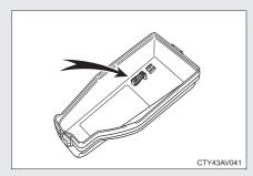
Only type A fuse can be removed using the pullout tool.
