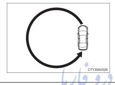
When "C" appears on the display, drive the vehicle at 5 mph (8 km/h) or less in a circle until a direction is displayed.
