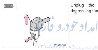
Unplug the connector while depressing the lock release.
