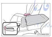
Slide the console box lid forward as needed. Slide the lid forward while pulling up the lever.
