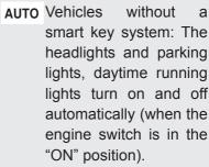
Vehicles with a smart key system: The headlights, parking lights, daytime running lights and so on turn on and off automatically (when the "ENGINE START STOP" switch is in IGNITION ON mode).
