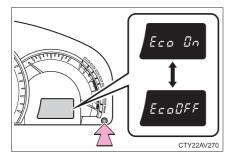
Eco Driving Indicator Light and current fuel consumption gauge can be activated or deactivated
