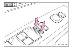
Shift the shift lever to P or N, and press and hold the driver's door lock switch ( or r) for approximately 5 seconds and then release.
