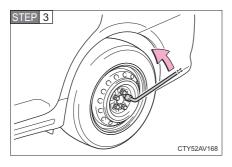
Slightly loosen the wheel nuts (one turn).
