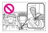
• Check that the shift lever is securely set in P. The engine may not start if the shift lever is displaced out of P.
