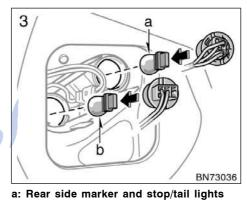
3. Install the bulb base into the mounting hole by turning it clockwise.
