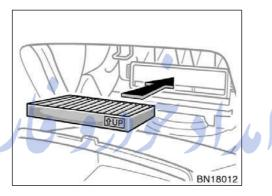
When inserting the filter in the filter outlet, keep the arrow pointing up.
