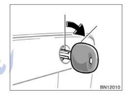
To open the trunk lid from the outside, insert the master key and turn it clockwise.
