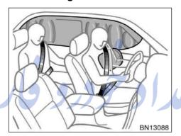
The SRS (Supplemental Restraint System) side airbags and curtain shield airbags are designed to provide further protection for the driver, front passenger and rear outside passengers in addition to the primary safety protection provided by the seat belts.
