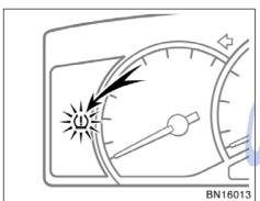
When initializing the system, make sure the low tire pressure warning light blinks three times. If the warning light does not blink three times, initializing will be failed and the tire pressure warning system will
