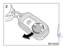
2. Remove the discharged transmitter battery.
