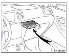
The air conditioning filter is behind the glove box.
