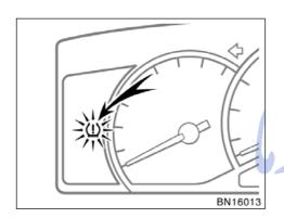
not blink when you push and hold the reset switch, have the low pressure warning system checked at your Toyota dealer. When the warning light blinks once every
