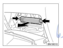
3. Remove the filter cover while pushing in both ends of the cover.
