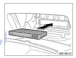
When inserting the filter in the filter outlet, keep the arrow pointing up.
