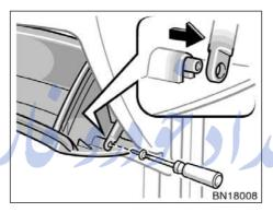
Open the glove box. Remove the 2. screw with a Phillips-head screw-driver and slide off the damper as shown.
