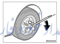
9. Lower the vehicle completely and tighten the wheel nuts.
