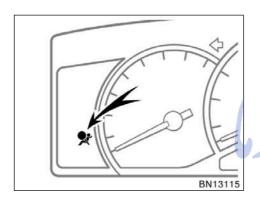
This indicator comes on when the ignition key is turned to the "ON" position. It goes off after about 6 seconds. This means the SRS side airbags are operating properly.
