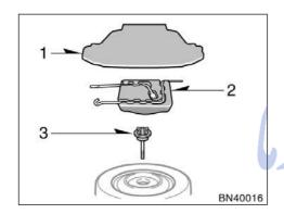
When storing the spare tire, put it in place with the outer side of the wheel facing up. Then secure the tire by repeating the above removal steps in reverse order to prevent it from flying forward during a collision or sudden braking.
