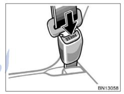
4. To remove the convertible seat, press the buckle release button and allow the belt to retract completely. The belt will move freely again and be ready to work for an adult or older child passenger.
