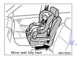
• A forward-facing child restraint system should be allowed to be installed on the front passenger seat only when it is unavoidable. Always move the seat as far back as possible even if the front passenger occupant classification indicator light indicates "OFF", because the front passenger airbag could inflate with considerable speed and force. Otherwise, the child may be killed or seriously injured.
