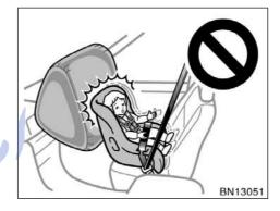
Never install a rear-facing child restraint system on the front passenger seat even if the front passenger occupant classification indicator light indicates "OFF". In the event of an accident, the impact of the rapid inflation of the front passenger airbag could cause death or serious injury to the child if the rearfacing child restraint system is installed on the front passenger seat.
