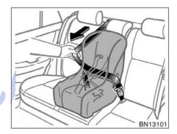
2. Fully extend the shoulder belt to put it in the lock mode. When the belt is then retracted even slightly, it cannot be extended.
