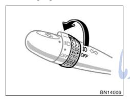
To turn on the front fog lights, twist the band of the headlight/turn signal lever. They will come on only when the headlights are on low beam.
