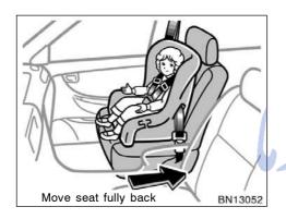
A forward-facing child restraint system should be allowed to be installed on the front passenger seat only when it is unavoidable. Always move the seat as far back as possible even if the front passenger occupant classification indicator light indicates "OFF", because the front passenger airbag could inflate with considerable speed and force. Otherwise, the child may be killed or seriously injured.
