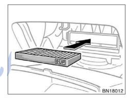
When inserting the filter in the filter outlet, keep the arrow pointing up.
