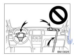
Do not put anything or any part of your baby on or in front of the dashboard or steering wheel pad that houses the front airbag system. They might restrict inflation or cause death or serious injury as they are projected rearward by the force of the deploying airbags. Likewise, the driver and front passenger should not hold objects in their arms or on their knees.
