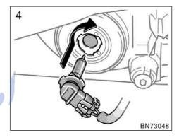
4. Install a new bulb and connector into the mounting hole.
