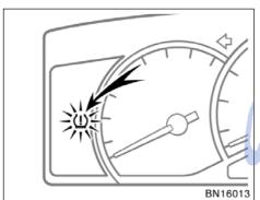
When initializing the system, make sure the low tire pressure warning light blinks three times. If the warning light does not blink three times, initializing will be failed
