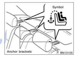
Use the anchor brackets on the luggage compartment to attach the top strap.
