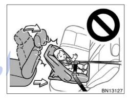
tem on the rear seat if it interferes with the lock mechanism of the front seats. Otherwise, the child or front seat occupant(s) may be killed or seriously injured in case of sudden braking or a collision.
