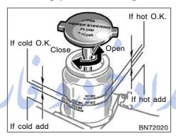
Check the fluid level through the reservoir. If necessary, add automatic transmission fluid DEXRONX II or III.
