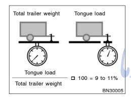
☐ The trailer cargo load should be distributed so that the tongue load is 9 to 11% of the total trailer weight, not exceeding the maximum of 68 kg (150 lb.). Never load the trailer with more weight in the back than in the front. About 60% of the trailer load should be in the front half of the trailer and the remaining 40% in the rear.
