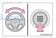
Vehicles with a manual transmission: Press the engine switch while turning the steering wheel left and right.
