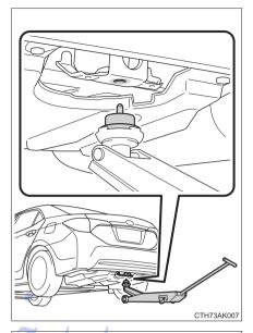
3 Before raising the vehicle, make sure that the floor jack is positioned so that the protrusion on the jack attachment fits securely into the hole of the jack point.
