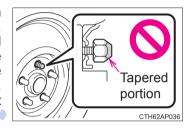
Never use oil or drease on the wheel bolts or wheel nuts. Oil and grease may cause the wheel nuts to be excessively tightened. leading to bolt or disc wheel damage. In addition, the oil or grease can cause the wheel nuts to loosen and the wheel may fall off, causing an accident and resulting in death or serious injury. Remove any oil or grease from the wheel bolts or wheel nuts.
