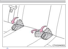
2 Pull the seatback lock release knob and fold the seatback down.
