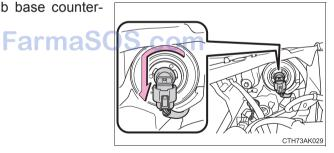
2 Pull the bulb out while pressing the lock release of the connector.
