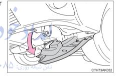
3 Unplug the connector while depressing the lock release.
