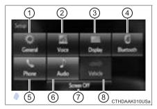
(4) Select to adjust the settings for registering, removing, connecting and disconnecting Bluetooth<sup>®</sup> devices. (→P. 339)
