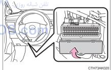
3 Remove the fuse with the pullout tool.
