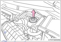
4 Add brake fluid slowly while checking the fluid level.
