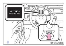
2 Press the "DISP" switch to select the item to be set, then press and hold the "DISP" switch.
