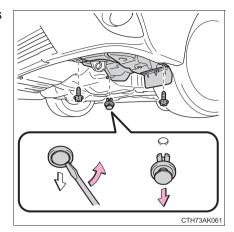
2 Partly remove the fender liner.
