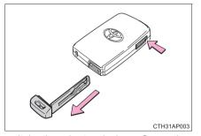
After using the mechanical key, store it in the electronic key. Carry the mechanical key together with the electronic key. If the electronic key battery is depleted or the entry function does not operate properly, you will need the mechanical key.  $(\rightarrow P. 535)$
