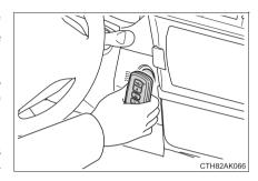
3 Vehicles with a drive monitor display: Firmly depress the brake pedal (continuously variable transmission) or clutch pedal (manual transmission) and check that the smart key system indicator light (green) turns on.
