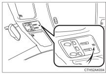
The vehicle's built in microphone is used when talking on the phone.
