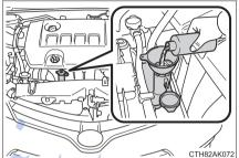
6 Start the engine to check that the radiator cooling fan operate and to check for coolant leaks from the radiator or hoses.
