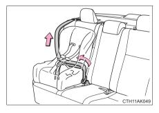
If the child restraint has a top tether strap, the top tether strap should be latched onto the top tether strap anchor.  $(\rightarrow P. 62)$
