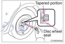
When replacing an aluminum wheel with a compact spare tire, tighten the wheel nuts until the tapered portion comes into loose contact with the disc wheel seat.
