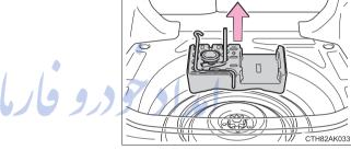
3 Loosen the center fastener that secures the spare tire.
