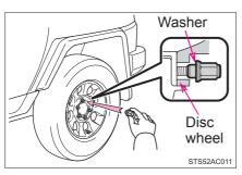
Tighten the nuts until the washer of the nut comes into loose contact with the disc wheel.
