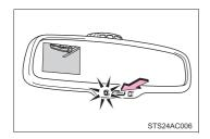
When the screen is displayed, press the AUTO button on the inside rear view mirror to switch the screen ON/OFF mode.
