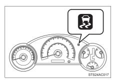
If the vehicle is in danger of slipping, or if the rear wheels (2WD models) or any of the drive wheels (4WD models) spins, the slip indicator flashes to indicate that VSC/TRAC (TRC) have been engaged.
