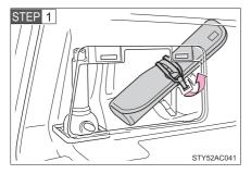
Remove the cover and loosen the strap.
