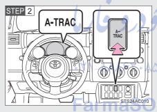
Press the A-TRAC switch to activate the system.
