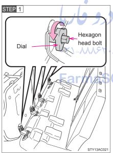
Loosen the bolts with a wrench at first and turn the dials by hand to remove them.
