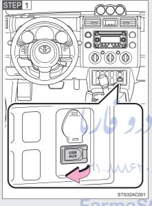
Open the cover and connect an iPod using an iPod cable.
