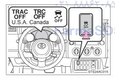
Press and hold the VSC OFF switch for more than 3 seconds while the vehicle is stopped to turn off both TRAC (TRC) and VSC.
