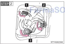
Turn the bulb bases counter-clockwise.
