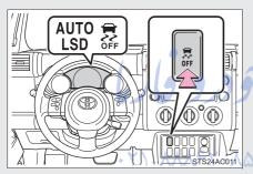
Press the VSC OFF switch to turn on the system.
