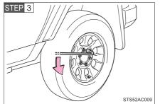
Slightly loosen the wheel nuts (one turn).
