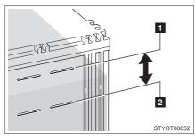
Check that the level is between the upper line and the lower line.
