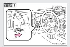
Hold the steering wheel and pull and hold the lever.
