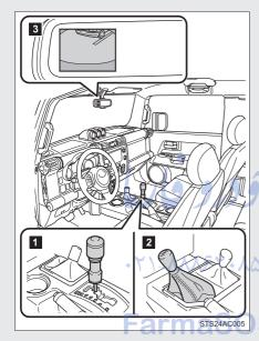
The rear view image is displayed on the inside rear view mirror when the shift lever is in the R.
