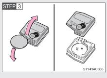
Open the case cover using a coin protected with tape etc. and remove the depleted battery.
