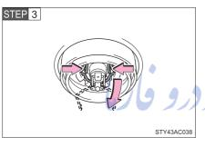
Release the bulb retaining spring.
