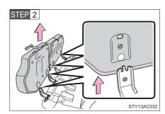
Separate the bottom cushion from the hinge.
