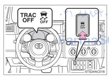
Press the VSC OFF switch for more than 3 seconds while the vehicle is stopped to turn off both TRAC and VSC.
