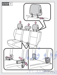
Stow the seat belt buckles and remove the head restraints.
