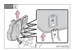
Separate the bottom cushion from the hinge.
