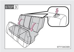
Push the lock release button and fold down the seatback.
