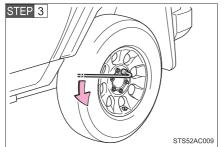
Slightly loosen the wheel nuts (one turn).
