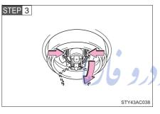
Release the bulb retaining spring.
