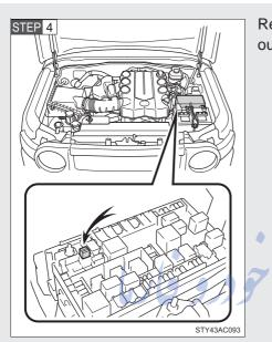
Remove the fuse with the pullout tool.
