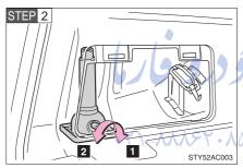
Loosen and remove the jack.
