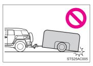
No matter which class of tow hitch applies, for a more safe trailer hookup, the trailer ball setup must be the proper height for the coupler on the trailer.
