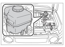
The brake fluid level should be between the MAX and MIN lines. on the reservoir.
