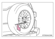
Turn the hold-down nuts counterclockwise with the wheel nut wrench and remove them.
