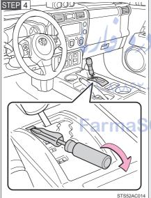
Pry the cover up with a flathead screwdriver or equivalent.
