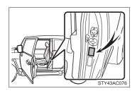
For the GAWR, see the Certification Label. For the maximum load of the tire, see the load limit at maximum cold tire inflation pressure mentioned on the sidewall of the tire. (→P. 496)
