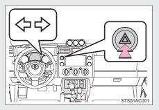
Press the switch to flash all the turn signal lights. To turn them off, press the switch once again.
