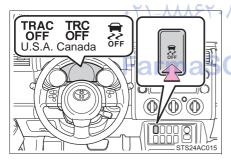
Press and hold the switch for more than 3 seconds while the vehicle is stopped to turn off TRAC (TRC) and VSC.
