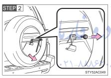
Remove the bolt which fixes the spare wheel cover using the wrench in the tool bag (→P. 454).
