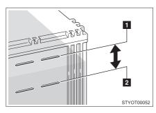
Check that the level is between the upper line and the lower line.
