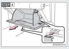
Then disconnect the claws at the bottom and remove the glove box.
