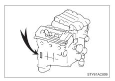
The engine number is stamped on the engine block as shown.
