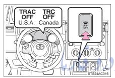
Quickly press and release the switch to turn off TRAC (TRC).
