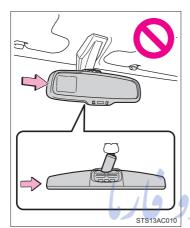
Do not push the mirror horizontally from the side. The mirror could fall off.
