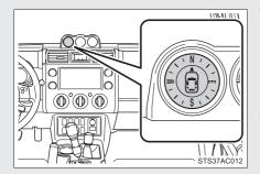
The compass points north for about 3 seconds after the engine switch is turned to the ON position, and then indicates the actual direction the vehicle facing.
