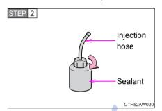
Connect the injection hose by screwing onto the sealant. As it is screwed in, the aluminum seal on the bottle will be torn.
