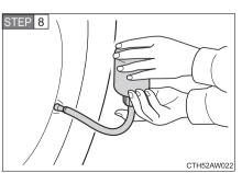
Inject the sealant that is in the bottle. Hold and tilt the bottle, then squeeze sealant out of the bottle as shown.
