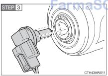
Replace the light bulb, and install
