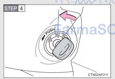
Vehicles without a smart entry & start system: Stop the engine by turning the engine switch to the "ACC" position.
