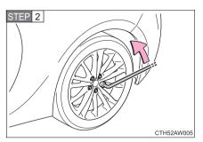
Slightly loosen the wheel nuts (one turn).
