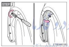
Remove the clip and partly remove the fender liner.
