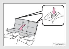
Press the seatback lock release buttons and fold the seatback down.
