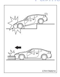
The SRS front airbag may be activated when the vehicle sustains a hard impact in the undercarriage area from the road surface (such as when the vehicle plunges into a deep ditch, is severely impacted or knocked hard against an obstacle on the road such as a curb).
