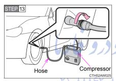
Connect the air compressor hose by threading it on the valve.
