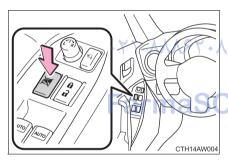
Press the switch down to lock the passenger window glasses.
