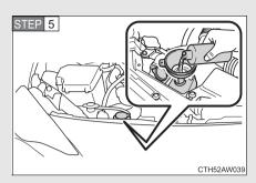
Add engine coolant if necessary.
