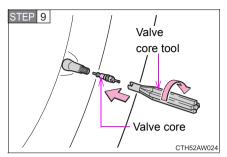
Remove the injection hose from the valve and screw the valve core in the valve securely by turning it clockwise with the valve core tool.
