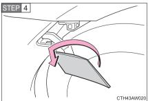
Pull out the lamp and turn the lens counterclockwise.
