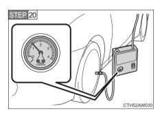
Read the inflation pressure on the pressure gauge.
