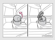
The ashtray can be installed in the cup holder. ( $\rightarrow$ P. 264)
