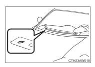
Headlight control sensor is located on the passenger's side.
