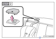
Remove the anchor bracket cover.
