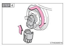
Turn and secure the bulb. Install the connector.
