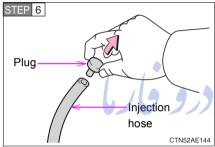
Remove the plug from the injection hose.
