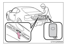
Press the button to unlock the trunk.
