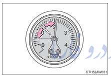
If the pressure is 130 kPa (1.3 kgf/cm<sup>2</sup> or bar, 19 psi) or above, fill the tire with air using the compressor until the specified inflation pressure is reached.
