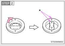
Turn the upper knob of each retaining hook (clip) to secure the floor mats in place.
