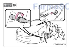
After driving about 10 minutes, pull your vehicle over in a safe place and reconnect the compressor.
