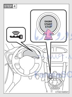
Press the "ENGINE START STOP" switch.
