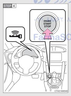
Press the "ENGINE START STOP" switch.
