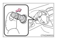
Turn off the engine with the light switch in **AUTO** or off, and pull the light switch toward you and release it. The low beam headlights will turn on for about 30 seconds to light up the area around the vehicle.
