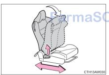
Lift the seatback angle adjustment lever.
