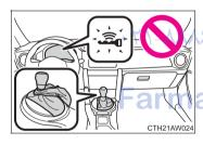
Vehicles with an automatic transmission: Check that the shift lever is securely set in P. The engine may not start if the shift lever is displaced out of P. The smart entry & start system indicator light (green) will flash quickly.
