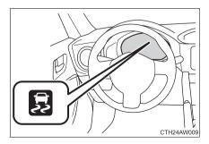
The slip indicator light will flash while the TRC (brake LSD function)/VSC systems are operating.
