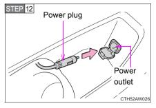
Connect the compressor power plug to the power outlet.
