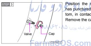
Position the nail or screw that has punctured the tire at the bottom, in contact with the ground. Remove the cap from the valve.
