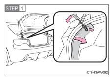
On some models, remove a clip and partly remove the cover.
