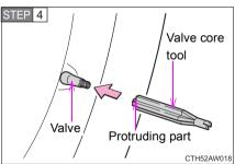
Bring the protruding part of the valve core tool into contact with the valve to discharge air.
