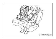
Put children in the REAR seat properly restrained at all times in a child restraint device or in a seat belt, whichever is appropriate for the child's age, height and weight. The SRS airbag deploys with considerable speed and force and can injure or even kill children, especially if they are not restrained or improperly restrained. Because children are lighter and weaker than adults, their risk of being injured from deployment is greater.
