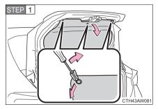
Vehicles with a trunk panel cover: Remove the trunk panel cover clips and partly remove the trunk panel cover.
