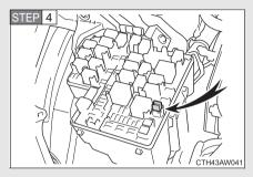
Remove the fuse with the pullout tool.
