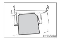
Make sure that the rear floor mats are installed in the correct position. If a floor mat is positioned incorrectly, it may interfere with the seat rail or other parts when a front seat is moved forward or backward, damaging the vehicle or floor mat.
