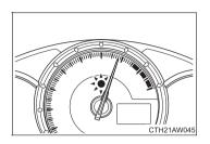
When the set engine speed is reached the REV indicator comes on and a buzzer sounds to inform the driver. ( $\rightarrow$ P. 205)
