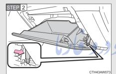
Open the glove box. Slide off the damper.
