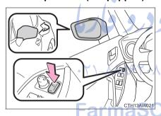
Press the switch to fold the mirrors.
