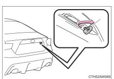
Turn the mechanical key clockwise to open.
