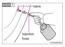
Connect the injection hose to the valve.
