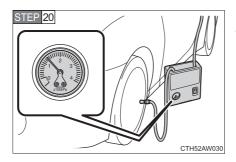
Read the inflation pressure on the pressure gauge.
