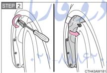
Remove the clip and partly remove the fender liner.
