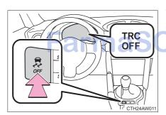
To turn the TRC system off, quickly press and release the button.
