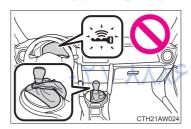
Vehicles with an automatic transmission: Check that the shift lever is securely set in P. The engine may not start if the shift lever is displaced out of P. The smart entry & start system indicator light (green) will flash quickly.
