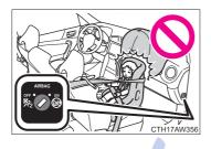
Never use a rear-facing child restraint system on the front passenger seat when the airbag manual on-off switch is on. (→P. 155)
