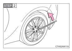
Slightly loosen the wheel nuts (one turn).
