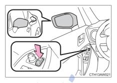
Press the switch to fold the mirrors.
