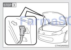
Hold the hood open by inserting the supporting rod into the
