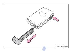
To take out the mechanical key, slide the release lever and take the key out.
