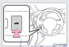
Press and hold the opener switch to release the trunk lid.
