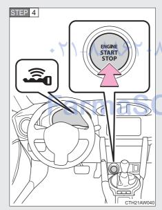
Press the "ENGINE START STOP" switch shortly and firmly.
