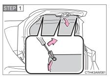
Vehicles with the trunk panel cover: Remove the trunk panel cover clips and partly remove the trunk panel cover.
