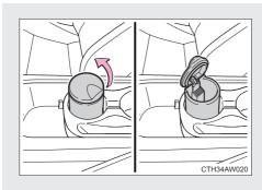
The ashtray can be installed in the cup holder. ( $\rightarrow$ P. 291)
