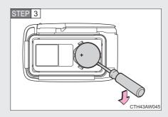
Remove the depleted battery.
