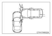
The vehicle is involved in a side-on impact in an area outside the vicinity of the passenger compartment.
