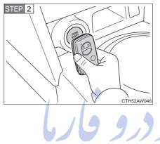
Touch the Toyota emblem side of the electronic key to the "ENGINE START STOP" switch.
