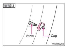
Position the nail or screw that has punctured the tire at the bottom, in contact with the ground. Remove the cap from the valve.
