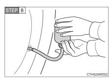
Inject the sealant that is in the bottle. Hold and tilt the bottle, then squeeze sealant out of the bottle as shown.
