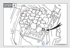
Remove the fuse with the pullout tool.
