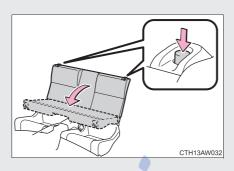
Press the seatback lock release buttons and fold the seatback down.
