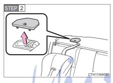
Remove the anchor bracket cover.
