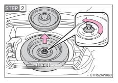
Remove the cover and loosen the center fastener that secures the spare tire.
