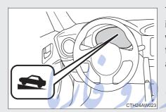
The hill-start assist control ON indicator will be illuminated when system is enabled and flash while the system is operating.
