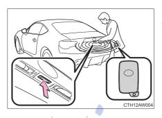
Press the button to unlock the trunk.
