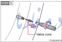
Pull out the valve core by turning it counterclockwise using the valve core tool.
