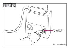
Turn the compressor switch "ON" and fill the tire with air until the specified inflation pressure is reached.
