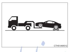
Vehicles with an automatic transmission: Use a towing dolly under the rear wheels.
