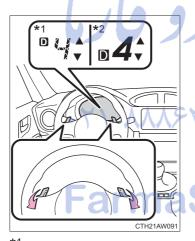
Temporary manual mode driving can be changed to by operating the paddle shift switches while the shift lever is in the D position.
