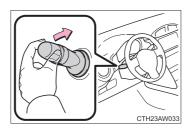
Turn off the engine with the light switch in **AUTO** or off, and pull the light switch toward you and release it. The low beam headlights will turn on for about 30 seconds to light up the area around the vehicle.
