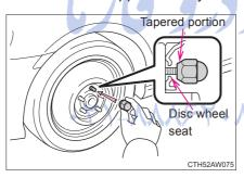
Vehicles with a compact spare tire: Tighten the wheel nuts until the tapered portion comes into loose contact with the disc wheel seat.
