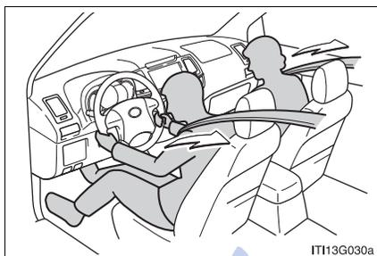
The pretensioner helps the seat belt to quickly restrain the occupant by retracting the seat belt when the vehicle is subjected to certain types of severe frontal collision or side collision (vehicles with SRS side airbags and curtain shield airbags).
