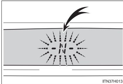
If the direction display on the compass flashes, circling calibration needs to be performed.
