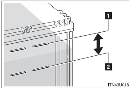
Check that the level is between the upper and lower lines.
