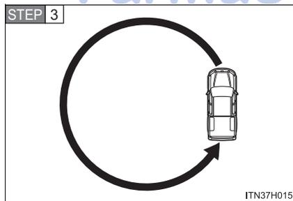
Drive the vehicle at 8 km/h (5 mph) or less in a circle until a direction is displayed.
