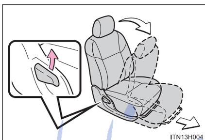
Pull the seatback angle adjustment lever and fold down the seatback. The seat will slide forward.
