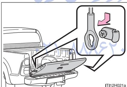
Release the brackets on the support cables from the lugs on both sides as shown in the illustration.
