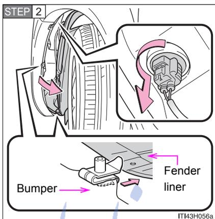
Partly remove the fender liner and turn the bulb base counter-clockwise.
