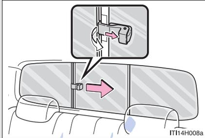
To open the back window, push the lock release lever and slide the back window.
