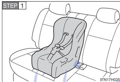
Place the child restraint system on the rear seat facing the front of the vehicle.
