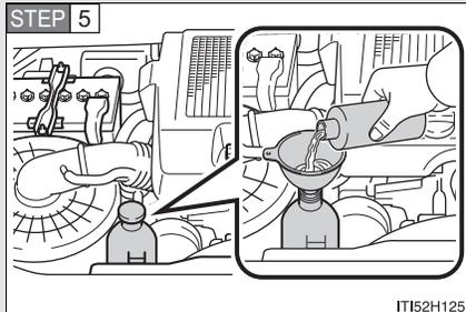
Add engine coolant if necessary.
