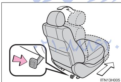
Depress the release pedal and fold down the seatback. The seat will slide forward.
