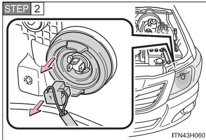
Unplug the connector and remove the rubber cover.
