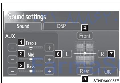
**1 2 3** Touch “-” or “+” to adjust the treble, mid or bass to a level between -5 to 5.
