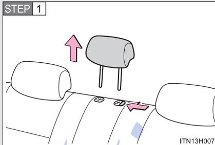
Remove the center head restraint.
