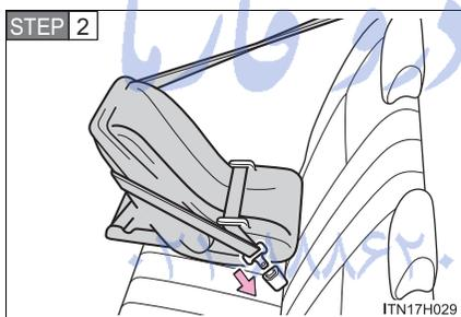
Run the seat belt through the child restraint system and insert the plate into the buckle. Make sure that the belt is not twisted. Keep the lap portion of the belt tight.
