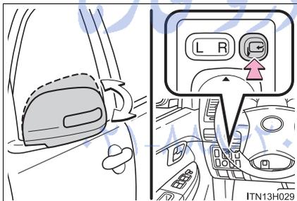
Press the switch to fold the mirrors.
