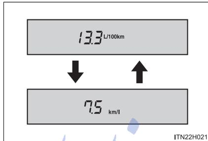
Unit for only the fuel consumption rate can be interchanged.
