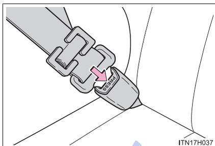
2-point type seat belt (if equipped): Push the buckle release button.
