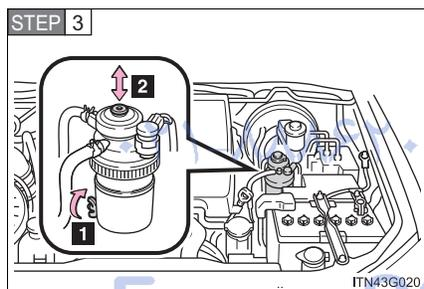
**1** Turn the drain plug counter-clockwise about 2 to 2 1/2 turns.
