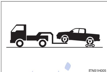
Vehicles with automatic transmission: Use a towing dolly under the rear wheels.
