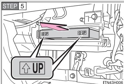
Remove the filter and replace it with a new one.
