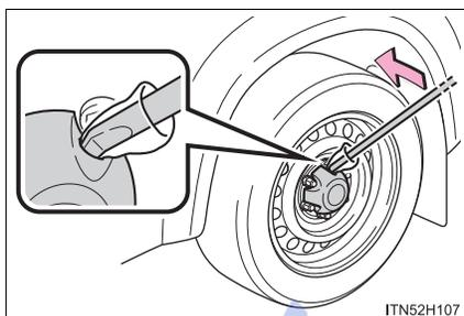
Pry off the wheel ornament, using the beveled end of the wheel nut wrench as shown.
