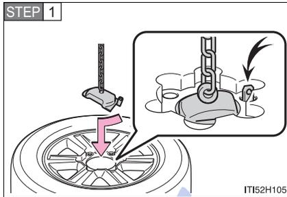
Lay down the tire with the outer side facing up, and hook the holding bracket as shown in the illustration.
