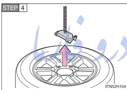
Remove the holding bracket and pull out the spare tire.
