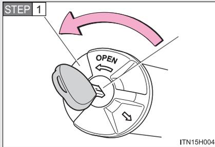
To unlock the fuel tank cap, insert the key and turn it counterclockwise.
