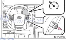
2 Accelerate or decelerate the vehicle to the desired speed, and push the lever down to set the speed.
