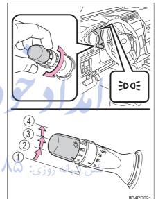
(4) **AUTO** Vehicles without a smart entry & start system: The head(if equipped) lights, front position lights, daytime running lights (→P. 284)
