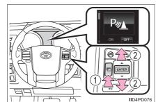
Press the "ENTER" switch to change to "ON". The Toyota parking assistsensor indicator will be dis-
