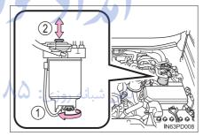
3 After draining, retighten the drain plug. Do not use a tool.
