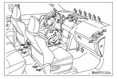
Adjusting the position of and opening and closing the air outlets
