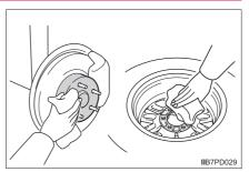
2 Install the spare tire and loosely tighten each nut by hand to approximately the same amount.
