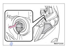
2 Unplug the connector while pushing the lock release.
