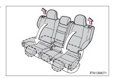
2 Pull the seat lock release lever on the back and swing the whole seat up and forward.
