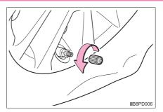
6 Remove the air release cap from the hose.
