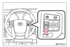
2 Press the "ENTER" switch upwards or downwards until "2ND START" appears.
