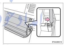
3 Push in each side of the glove box to disconnect the claws.
