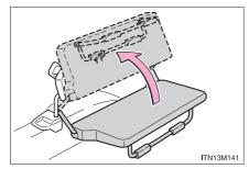
2 Take the holding strap of its pocket on the back of the seatback and secure the seat hooking the strap onto the hook in the back of the seat cushion.
