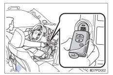
Press the engine switch within 10 seconds of the buzzer sounding, keeping the brake pedal depressed.
