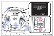
3 Press the "ENTER" switch to change to "ON".
