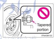
• Never use oil or grease on the wheel bolts or wheel nuts.
