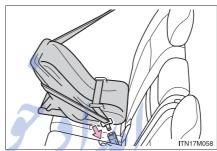
Install a locking clip near the tab of the lap and shoulder belt by inserting the lap and shoulder webbing through the recesses of the locking clip. Buckle the belt again. If the belt has any slack, release the buckle and reinstall the locking clip.
