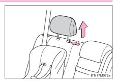
2 Open the anchor bracket cover, latch the hook onto the anchor bracket and tighten the top strap.
