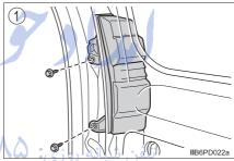
2 Close the back door half way and remove the lamp
