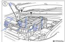
2 Raise the front of the engine cover and then pull the cover to detach it from the bracket on the rear bar as shown in the illustration.
