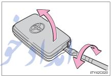
3 Remove the depleted battery. Insert a new battery with the "+" terminal facing up.
