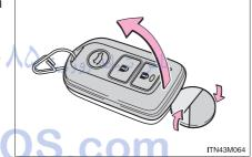
Remove the depleted battery using the tip of a ball-point pen or a similar pointed object.
