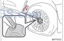
3 Slightly loosen the wheel nuts (one turn).
