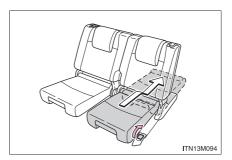
2 Pull the seatback lock release lever and fold them down.
