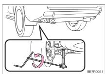
4 Firmly tighten each nut two or three times in the order shown in the illustration.
