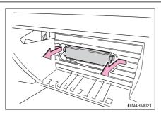
The "↑UP" marks shown on the filter should be pointing up.
