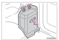
2 Take out the emergency tire puncture repair kit.
