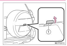
2 Remove the bolt which fixes the spare tire cover.
