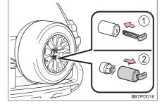
2 Turn the hold-down nuts counterclockwise with the wheel nut wrench and remove them.
