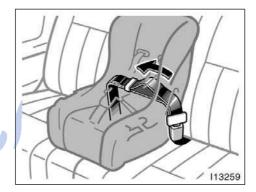
While pressing the convertible seat firmly against the seat cushion and seatback, tighten the lap belt by pulling its free end to hold the convertible seat securely.
