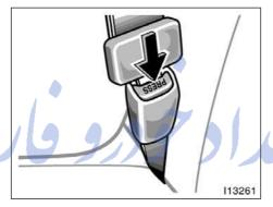
3. To remove the convertible seat, press the buckle-release button.
