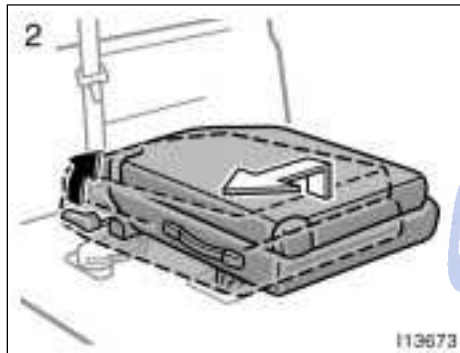
2. Unlock the seat cushion and slide the whole seat to the rear-most position while pulling up the handle.
