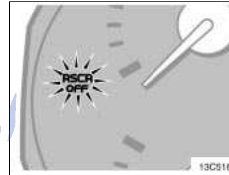
Roll sensing of curtain shield airbags off indicator light
