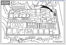
Remove the fuse with the pullout tool.
