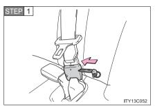
To release the hooked tab, insert the mechanical key into the hole on the buckle with the light gray buckle release button.
