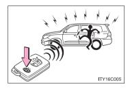
When (() is pressed for longer than about one second, the headlights/tail lights/emergency flashers will flash, the front and rear interior lights will come on, and an alarm will sound for about 60 seconds to deter any person from trying to break into or damage your vehicle.
