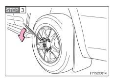
Slightly loosen the wheel nuts (one turn).
