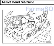
When a front seatback receives a strong impact, the head restraint moves slightly forward and upward to help reduce the risk of whiplash on the seat occupant.
