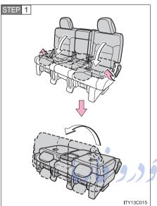
Fold down the seatback while pulling the seatback angle adjustment lever, and swing the whole seat up and forward.
