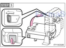
Lift the seats sideward while pulling the seat leg lock release levers.
