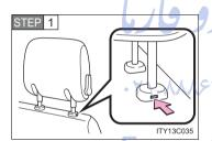
Push a flathead screwdriver into the slot. The slot is located on the left side of the left head restraint anchor.
