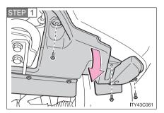
Remove the fender liner bolts and clip and remove the fender liner.
