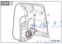
Turn the bulb bases counter-clockwise.
