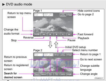
If  $\bigcirc$  appears on the screen when you select an icon, the operation relevant to that control is not permitted.
