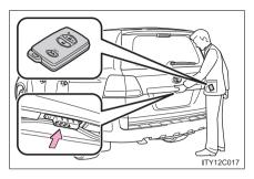
Press the unlock button to unlock the back door.
