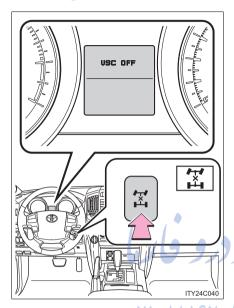
Push the center differential lock/ unlock switch to turn off VSC system.
