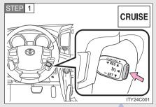
Press the "ON-OFF" switch to operate the cruise control.
