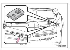
Press the lock button to lock the back door.
