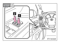
Shift the shift lever to "P" or "N", press and hold the driver's door lock switch (1 or 2) for 5 seconds then release.
