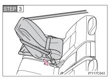
Run the seat belt through the infant seat/convertible seat and insert the plate into the buckle. Make sure that the belt is not twisted.
