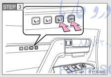
While pressing the "SET" button, press button "1", "2" or "3" until the signal beeps.
