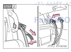
Hook the holding strap to the assist grip and secure the seat by pulling its free end.
