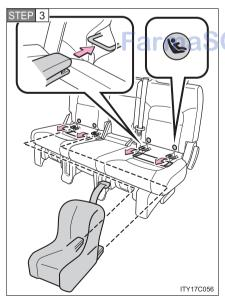
Latch the buckles onto the anchors.
