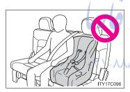
When using the left side lower anchors for the child restraint system, do not sit in the center seat. Seat belt function may be impaired, such as being positioned overly high or loose-fitting, which may result in death or serious injury in the event of a collision.
