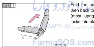
Fold the seatback forward and then back to the 1st lock position (most upright position) until it locks into place.
