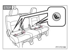
Take off the covers between the seat cushion and seatback, then confirm the position of the lower anchors below the symbol in the seatback.
