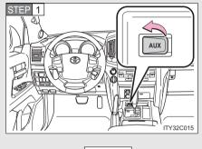
Connect the portable audio device.
