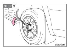
Slightly loosen the wheel nuts (one turn).
