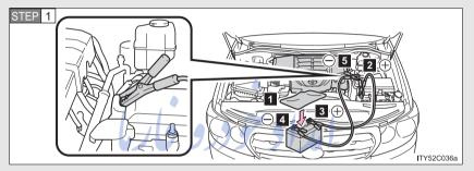
Connecting the jumper cables.
