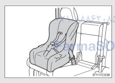
Seat belts equipped with a child restraint locking mechanism (ALR/ELR belts except driver's seat belt) (→P. 70)
