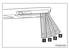
The display angles change as follows each time TILT is pressed.
