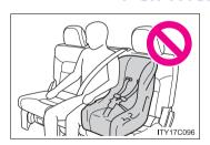
1 When using the left side lower anchors for the child restraint system, do not sit in the center seat. Seat belt function may be impaired, such as being positioned overly high or loose-fitting, which may result in death or serious injury in the event of a collision.
