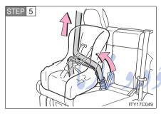
While pushing the convertible seat into the seat, allow the shoulder belt to retract until the convertible seat is securely in place.
