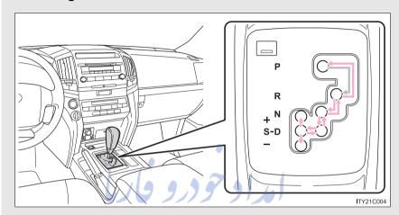
While the "ENGINE START STOP" switch is in IGNITION ON mode, depress the brake pedal and move the shift lever.
