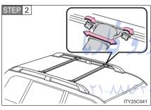
Slide the cross rails to the appropriate position for loading luggage and turn the knobs clockwise to tighten the cross rails securely.
