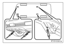
If your Toyota is transported by a flat bed truck, it should be tied down at the locations shown in the illustration. When attaching the hooks to the rear of the vehicle, make sure to attach them to the inside of the vehicle.
