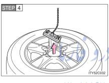
Pull out the spare tire and remove the holding bracket.
