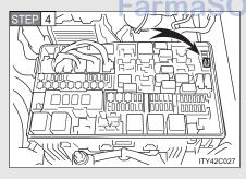
Remove the fuse with the pullout tool.
