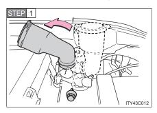
For the left side only: Remove the securing bolt and move the washer fluid filler opening.
