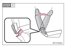
Fold the seatback while pulling the seatback angle lever. Return the seatback and secure it at the first lock position.  $(\rightarrow P. 54)$
