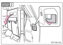
Unlock the seats by pulling the stowed seat lock release levers and lower the seats to its original position.
