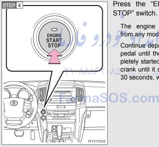
Press the "ENGINE START STOP" switch.
