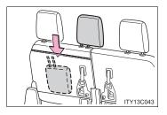
Open the zipper on the back of the third seat and stow the head restraint inside.
