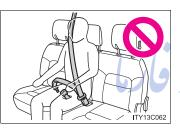
Do not use the third center seat belt with either buckle released. Fastening only one of the buckles may result in death or serious injury in case of sudden braking, sudden swerving or a collision.
