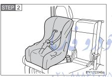
Place the child restraint system on the second or third seat facing the front of the vehicle.
