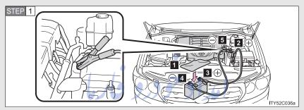
Connecting the jumper cables.
