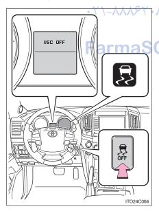
Push and hold the button for more than 3 seconds while the vehicle is stopped to turn off Active TRAC and VSC.
