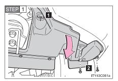
Remove the fender liner bolts, loose the fender liner nut and remove the fender liner.
