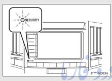
The indicator light flashes after the "ENGINE START STOP" switch has been turned OFF to indicate that the system is operating.
