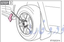
Slightly loosen the wheel nuts (one turn).
