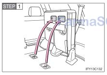
Remove the seat hook covers from the floor and install them into the back of the seat cushion.
