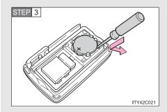
Remove the depleted battery.
