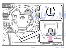
Press and hold the tire pressure warning reset switch until the tire pressure warning light blinks slowly 3 times and the message "TIRE PRESSURE RESET PROCEEDING" appears on the multi-information display.
