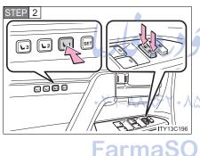
While pressing the desired button ("1", "2", or "3"), press the lock or unlock side on the door lock switch until the signal beeps.
