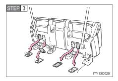
Remove the seat hook covers from the back of the seat cushion, and install them on the seat hooks.
