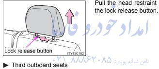
Pull the head restraint up while pressing
