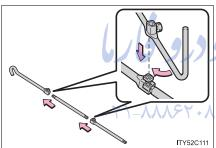
Assemble the jack handle extension bar and the jack handle bar and tighten the bolts.
