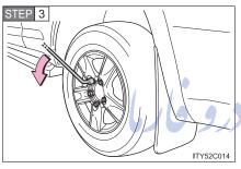
Slightly loosen the wheel nuts (one turn).
