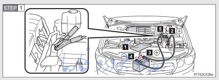
Connecting the jumper cables.
