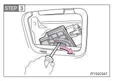
Push the lever for the back door motor, open the back door.
