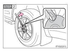
Pry off the wheel ornament, using the beveled end of the wheel ornament remover as shown.
