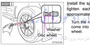
Install the spare tire and loosely tighten each nut by hand to approximately the same amount.
