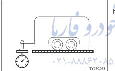
The load placed on the trailer hitch ball. ( $\rightarrow$ P. 240)
