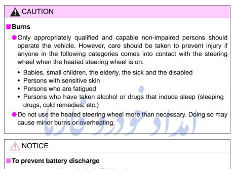
Turn the switch off when the engine is not running.
