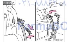
Hook the holding strap to the assist grip and secure the seat by pulling its free end.
