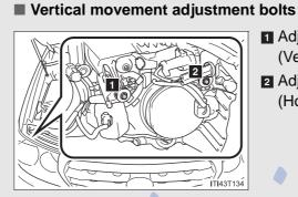
Adjustment bolt A (Vertical adjustment)
