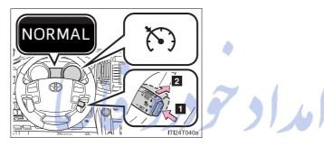
Press the "ON-OFF" button to activate the cruise control. Press the button again to deactivate the cruise control.
