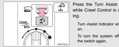
Press the Turn Assist switch while Crawl Control is operat-
