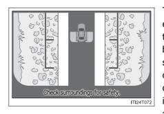
The image from both side cameras is displayed. Use this monitor to help check the area on both sides of the vehicle at the same time, and to check for objects near the tires or the sides of the vehicle. Guidelines showing an image of the vehicle width and the position of the rear tires are displayed.
