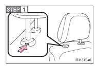
Push a flathead screwdriver into the slot. The slot is located on the right side of the right head restraint anchor.
