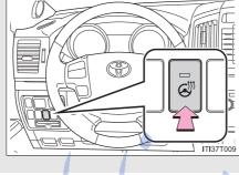
The indicator light comes on when the heater is operating.
