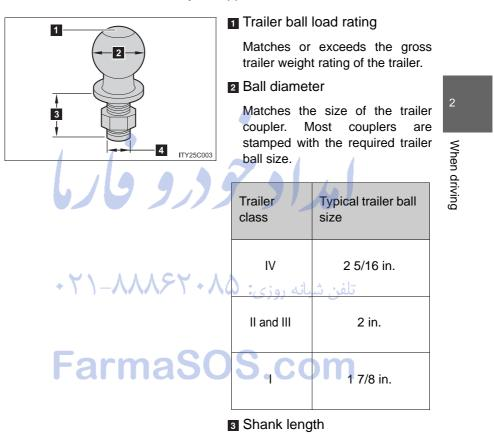
Protrudes beyond the bottom of the lock washer and nut by at least 2 threads.
