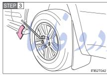
Slightly loosen the wheel nuts (one turn).
