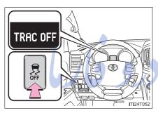
Quickly push and release the button to turn off Active TRAC.
