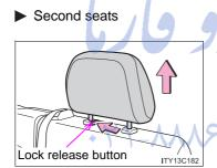
Pull the head restraint up while pressing the lock release button.
