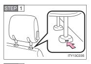
Push a flathead screwdriver into the slot. The slot is located on the left side of the left head restraint anchor.
