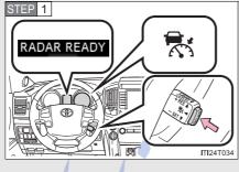
STEP 2 SET George Control of the second seco Press the "ON-OFF" button to activate the cruise control.
