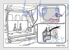
Remove the cover. Hold the warning reflector with the bands.
