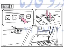
While pressing the desired button ("1", "2", or "3"), press the lock or unlock side on the door lock switch until the signal beeps.
