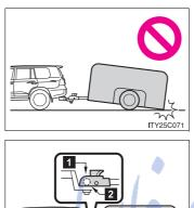
No matter which class of tow hitch applies, for a more safe trailer hookup, the trailer ball setup must be the proper height for the coupler on the trailer.
