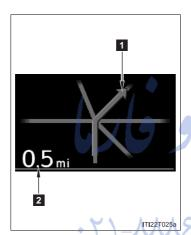
The turn-by-turn navigation appears only while route guidance of the navigation system is being performed. When a turn approaches, the distance to the turn and the turn direction are displayed.
