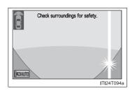
If a bright light, such as sunlight reflected off the vehicle body, is picked up by the camera, a smear effect<sup>\*</sup> characteristic to the camera may occur.
