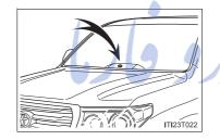
The sensor may not function properly if an object is placed on the sensor, or anything that blocks the sensor is affixed to the windshield.
