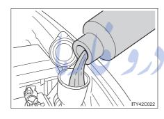
If any washer does not work or the warning message appears on the multi-information display, the washer tank may be empty. Add washer fluid.
