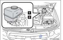
The brake fluid level should be between the "MAX" and "MIN" lines on the tank.
