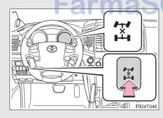
Lock the center differential when your vehicle's wheels get stuck in a ditch or when driving on a slippery or bumpy surface.
