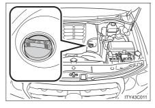
If the oil level is below or near the low level mark, add engine oil of the same type as already in the engine. ( $\rightarrow$ P. 669)
