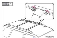
Turn the knobs counterclockwise to release the cross rails.
