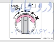
Operate the Multi-terrain Select mode select switch during Multi-terrain Select control to select a mode.
