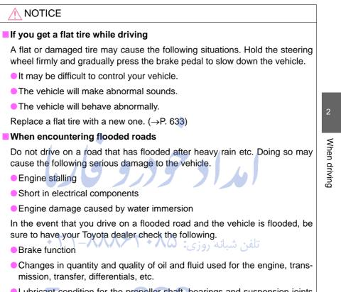
Lubricant condition for the propeller shaft, bearings and suspension joints (where possible) and the function of all joints, bearings, etc.
