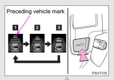
Pressing the button changes the vehicle-to-vehicle distance as follows:
