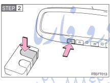
Press and hold one of the HomeLink® buttons and the transmitter button. When the HomeLink® indicator light changes from a slow to a rapid flash, you can release both buttons.
