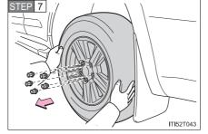
When resting the tire on the ground, place the tire so that the wheel design faces up to avoid scratching the wheel surface.
