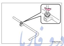
**1** Loosen the screw using a screwdriver.
