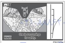
The minimum projected turning circle line is added to the no course lines mode.
