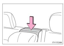
Lower the head restraint to the lowest position.
