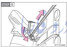
While pushing the child restraint system down into the seat, allow the shoulder belt to retract until the child restraint system is securely in place.
