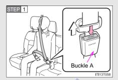
Push the release button on buckle A
