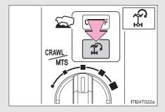
Press the Turn Assist switch while Crawl Control is operating.
