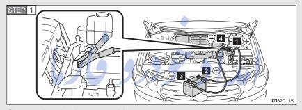
Connecting the jumper cables.
