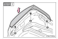
Open the back door and remove the nuts and lamp assembly.
