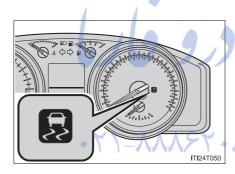
The slip indicator light flashes to indicate that the VSC/Trailer Sway Control/Active TRAC/hill-start assist control systems have been engaged.
