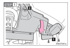
Remove the fender liner bolts, loose the fender liner nut and pull down the fender liner.
