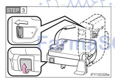
Pull the seat leg lock release levers.
