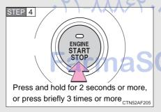
To stop the engine, press and hold the "ENGINE START STOP" switch for 2 consecutive seconds or more, or press it briefly 3 times or more in succession.
