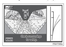
The projected course line is added to the minimum projected turning circle mode.
