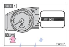
While the odometer is being displayed, press and hold the odometer/trip meter display change button to display the Eco Driving Indicator Light customization screen.
