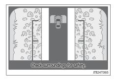
The image from both side cameras is displayed. Use this monitor to help check the area on both sides of the vehicle at the same time, and to check for objects near the tires or the sides of the vehicle. Guidelines showing an image of the vehicle width and the position of the front tires are displayed.
