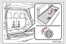
Remove the cover. Hold the warning reflector with the bands.
