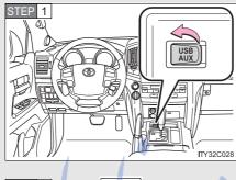
Open the cover and connect the portable audio device.
