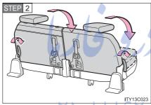
Push the seatback angle levers and fold the third seatbacks.
