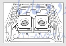
To hang the cargo net, use the cargo net hooks and rear tiedown hooks.
