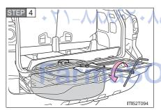
Lower the spare tire completely to the ground. تلفن شا
