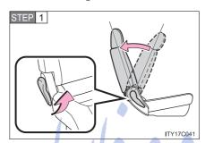
Fold the seatback while pulling the seatback angle lever. Return the seatback and secure it at the first lock position.  $(\rightarrow P. 59)$
