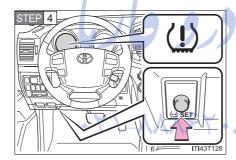
Press and hold the tire pressure warning reset switch until the tire pressure warning light blinks slowly 3 times and the message "TIRE PRESSURE RESET PROCEEDING" appears on the multi-information display.
