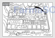
Remove the fuse with the pullout tool.
