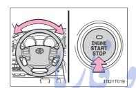
The green indicator light on the "ENGINE START STOP" switch will flash and a message will be shown on the multi-information display. Press the "ENGINE START STOP" switch again while turning the steering wheel left and right.
