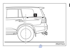
■ Hitch receiver pin hole position: 45.3 in. (1151 mm)
