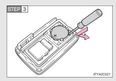
Remove the depleted battery.
