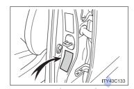
For the GAWR, see the Certification Label. For the maximum load of the tire, see the load limit at maximum cold tire inflation pressure mentioned on the sidewall of the tire.  $(\rightarrow P. 682)$
