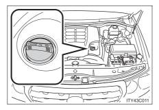
If the oil level is below or near the low level mark, add engine oil of the same type as already in the engine. ( $\rightarrow$ P. 671)
