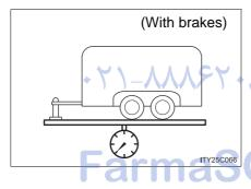
The maximum allowable gross trailer weight. The gross trailer weight is the sum of the trailer weight and the weight of the cargo in the trailer.
