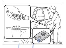
Grip the driver's door handle to unlock the door. Grip the passenger's door handle to unlock all the doors.\*
