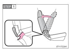
Fold the seatback while pulling the seatback angle lever. Return the seatback and secure it at the first lock position. (→P. 59)
