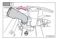
For the left side only: Remove the securing bolt and move the washer fluid filler opening.
