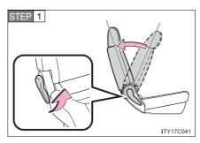
Fold the seatback while pulling the seatback angle lever.
