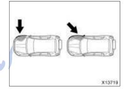
The SRS side airbag and curtain shield airbag system may not activate if the vehicle is subjected to a collision from the side at certain angles, or a collision to the side of the vehicle body other than the passenger compartment as shown in the illustration.
