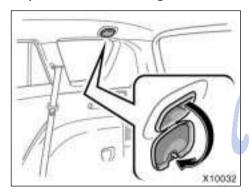
This is the hook to fix the separation net which is the option installment kit for Toyota dealer.
