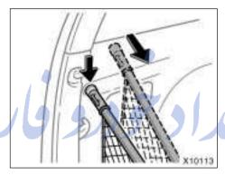
Compress the left end of the pipe, and fit it into the hole on the other side of the luggage compartment.
