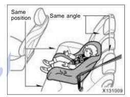
• When installing a child restraint system on the rear/second center position, adjust both seat cushions to the same position and align all seatbacks at the same angle. Otherwise, the child restraint system cannot be securely restrained and this may cause death or serious injuries in a collision.
