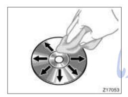
To clean a disc: Wipe it with a soft, lint-free cloth that has been dampened with water. Wipe in a straight line from the center to the edge of the disc (not in circles). Dry it with another soft, lint-free cloth. Do not use a conventional record cleaner or anti-static device.
