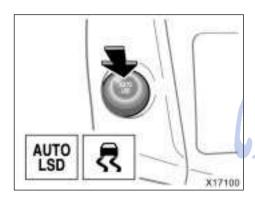
To activate the system, push the "AUTO LSD" switch with the vehicle stopped.
