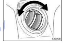
If air flow control is not satisfactory, check the side vents. The side vents may be ing opened or closed as shown.
