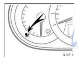
This indicator comes on when the ignition key is turned to the "ON" position. It goes off after about 6 seconds. This means the SRS front airbags are operating properly.
