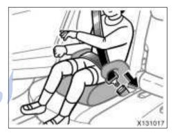
1. Sit the child on a booster seat. Run the lap and shoulder belt through or around the booster seat and across the child following the instructions provided by its manufacturer and insert the tab into the buckle taking care not to twist the belt.
