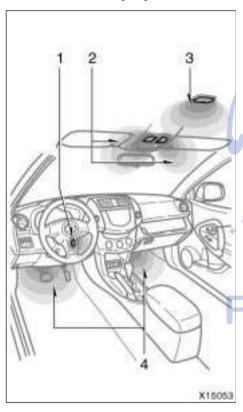
The following lights will come on when any of the side doors are opened. After all the side doors are closed, the lights remain on for about 15 seconds before fading out.
