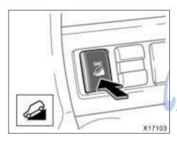
Push the "DAC" switch to turn the system on. The downhill assist control system indicator light will come on.
