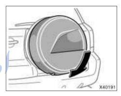
2. Attach the cover by hooking the 2 inner protrusions.
