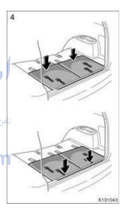
Push the seat on the front side against the floor and push the seat on rear side against the floor. Make sure it is locked securely.
