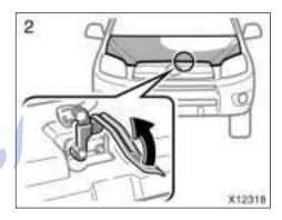
2. In front of the vehicle, pull up the auxiliary catch lever and lift the lood.
