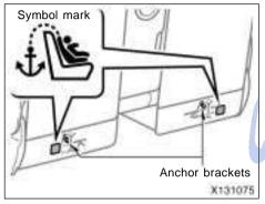
Use one anchor bracket on the roof and two anchor brackets on the rear/second seatbacks to attach the top strap.
