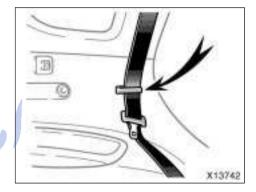
3. Make sure the outer seat belt passes through the hanger when folding the rear/second seat.
