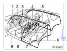
The SRS side airbag and curtain shield airbag system consists mainly of the following components, and their locations are shown in the illustration.
