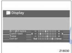
After adjusting the screen, push the "ENT" button or "DISPLAY" button to return to the previous screen.
