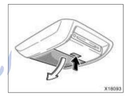
To open the display, push the lock release button.
