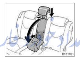
To use the armrest, lower the center head restraint. Pull the strap and pull the armrest down.
