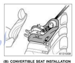
A convertible seat must be used in forward-facing or rear-facing position depending on the age and size of the child. When installing, follow the manufacturer's instructions about the applicable age and size of the child as FarmaSOS.com well as directions for installing the child restraint system.
