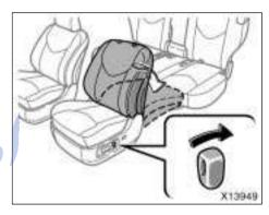
Move the seatback angle adjusting switch backward to flatten the seatξ γ back.
