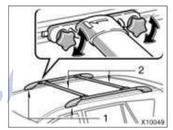
The roof luggage carrier consists of roof rails (1) attached to the roof and sliding cross rails (2).
