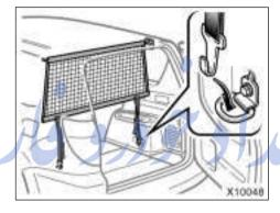
You can use the tie-down hooks to hook the claw of the separation net strap.
