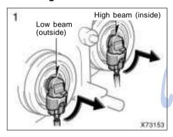
Open the hood. Turn the bulb base counterclockwise to the front of the vehicle as shown.
