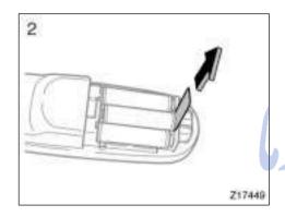
2. Remove the insulating sheet.
