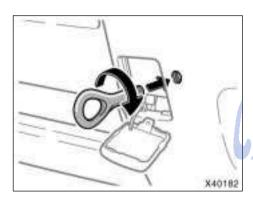
Use the front towing eyelet in the tool bag. Secure it to the hole on the bumper by turning clockwise. (For the tool bag location, see "—Required tools and spare tire" on page 326 in this Section.)
