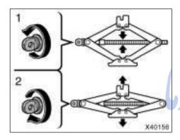
To remove the jack, turn the jack joint by hand.
