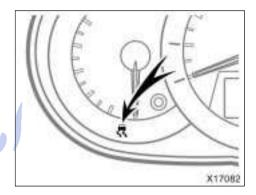
When the hill-start assist control system is operating, the slip indicator light flashes and the stoplights and high mounted stoplight are lit.
