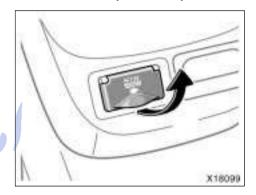
This power outlet is designed for use as a power supply for electric appliances in the vehicle.
