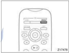
Operate the joystick up and down to select Brightness, Contrast, Tone, or Color and left and right to make adjustments.
