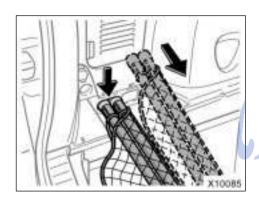
Compress the left end of the rear cargo net, and fit it into the other side of the luggage storage box.
