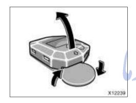
3. Open and remove the battery case cover using a coin.
