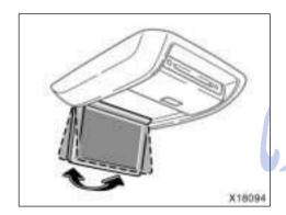
Pull the display down to an easily viewable angle (between  $90^{\circ}$  and  $125^{\circ}$ )
