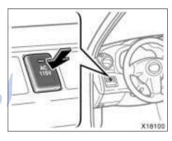
To use the power outlet, push the main switch on the instrument panel.
