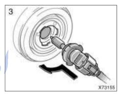
3. Pulg in a new bulb into the connector and install it into the mounting
