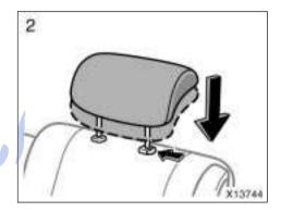
2. Lower the head restraint to the lowest position.
