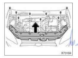
Before replacing the battery, remove the cover as shown.
