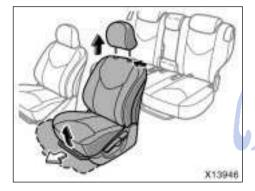
2. Remove the front head restraint. Hold the center of the lever and pull it up. Then slide the front seat further forward than the front-most lock position.
