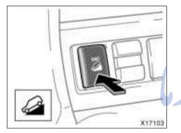
2. Push the "DAC" switch to turn the system on. The downhill assist control system indicator light will come on.
