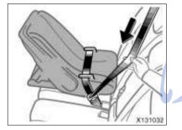
2. Fully extend the shoulder belt to put it in the lock mode. When the belt is then retracted even slightly, it cannot be extended.
