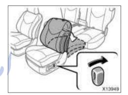
3. Move the seatback angle adjusting switch backward to flatten the seat-
