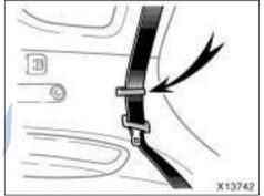
3. Make sure the outer seat belt passes through the hanger when folding the city rear/second seat.
