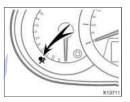
This indicator comes on when the ignition key is turned to the "ON" position. It goes off after about 6 seconds. This means the SRS side airbags and curtain shield airbags are operating properly.
