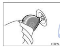
The engine immobilizer system is a theft prevention system. When you insert the key in the ignition switch, the transponder chip in the key's head transmits an electronic code to the vehicle. The engine will start only when the electronic code in the chip corresponds to the registered ID code for the vehicle.
