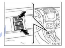
To turn on the seat heater, push the switches ("L" switch for the left front seat and "R" switch for the right front seat). At this time, the indicator light will illuminate to indicate the seat heater is operating.
