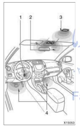
The following lights will come on when any of the side doors are opened. After all the side doors are closed, the lights remain on for about 15 seconds before fading out.
