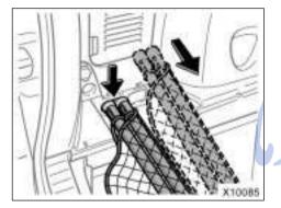
4. Compress the left end of the rear cargo net, and fit it into the other side of the luggage storage box.
