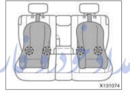
Lower anchorages for the child restraint systems complying with the FMVSS225 or CMVSS210.2 specifications are installed in the rear/second seat.
