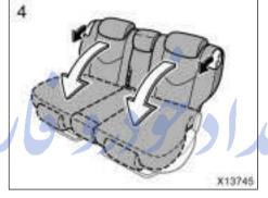
4. Pull down the seatback angle adjusting lever and fold down the seatback.
