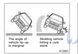
The curtain shield airbags may inflate if the angle of vehicle tip-up is marginal or if the skidding vehicle's tires hit a curb stone laterally as shown in the illustration.
