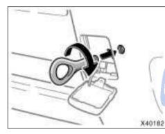
2. Use the front towing eyelet in the tool bag. Secure it to the hole on the bumper by turning clockwise. (For the tool bag location, see "—Required tools and spare tire" on page 356 in this Section.)
