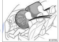
The SRS (Supplemental Restraint System) front airbags are designed to provide further protection for the driver and front passenger in addition to the primary safety protection provided by the seat belts.
