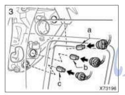
a: Rear side marker light b: Rear turn signal light c: Back–up light
