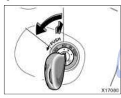
"START"—Starter motor on. The key will return to the "ON" position when released.
