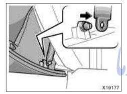
1. Open the glove box. Slide off the damper as shown.
