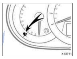
This indicator comes on when the ignition key is turned to the "ON" position. It goes off after about 6 seconds. This means the seat belt pretensioners are operating properly.
