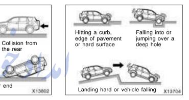
The SRS side and curtain shield airbags may deploy if a serious impact occurs to the underside of your vehicle. Some examples are shown in the illustration.
