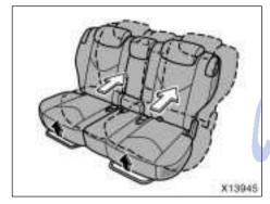
1. Hold the center of the lever and pull it up. Then slide the rear/second seats fully backward and pull it forward slightly until it locks.
