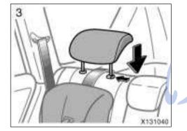
3. Insert the head restraint and push it down to the lock position.
