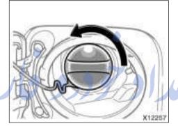
2. To remove the fuel tank cap, turn the cap counterclockwise. Pause -slightly before removing it. It is not unusual to hear a slight swoosh when the cap is opened.
