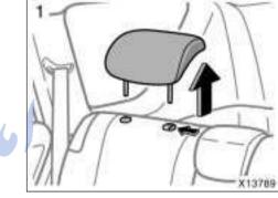
TO USE THE OUTSIDE ANCHOR BRACKET: A emove the head restraint.
