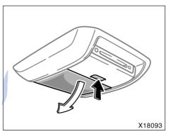
To open the display, push the lock release button.
