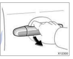
To open the back door, pull the handle. All the side doors and back door lock and unlock simultaneously with the driver's door.
