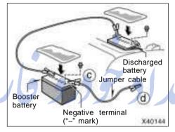
c. Connect the clamp of the negative (black) cable to the negative (-) terminal on the booster battery.
