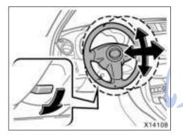
To adjust the steering wheel position, push down the lock release lever. Then tilt the steering wheel to the desired angle, push or pull it to the desired steering column length and return the lever to its original position.
