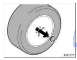
On some models—Before stowing the flat tire, remove the center wheel or  $\sim 1$ . Insert the hooks under the guides nament by pushing from the reverse side.
