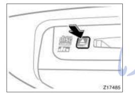
EJECTING THE DISC Push the "**≜**" button.
