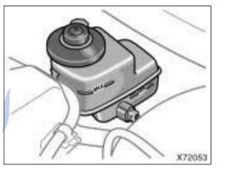
To check the fluid level, simply look at the see-through reservoir. The level should be between the "MAX" and "MIN" lines on the reservoir.
