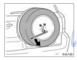
To remove the spare tire, turn the hold-down nuts counterclockwise with the wheel nut wrench and remove them.
