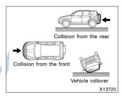
The SRS side airbags are not generally designed to inflate if the vehicle is involved in a front or rear collision, if it rolls over, or if it is involved in a low-speed side collision.
