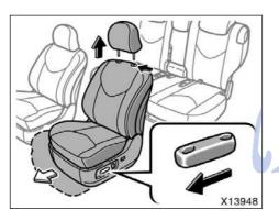
Remove the front head restraint. Push the seat position adjusting switch forward to slide the seat to the front-most position.
