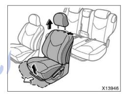
2. Remove the front head restraint.
