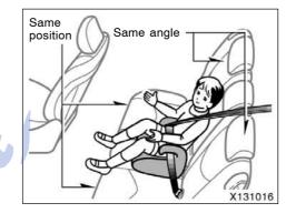
• When installing a child restraint system on the rear/second center position, adjust both seat cushions to the same position and align all seatbacks at the same angle. Otherwise, the child restraint system cannot be securely restrained and this may cause death or serious injuries in a collision.
