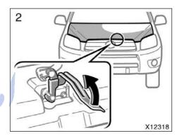
2. In front of the vehicle, pull up the auxiliary catch lever and lift the food.
