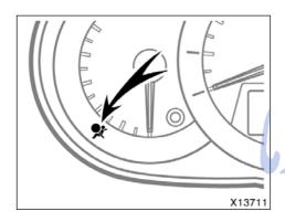
This indicator comes on when the engine switch is turned to the "ON" position. It goes off after about 6 seconds. This means the SRS side airbags and curtain shield airbags are operating properly.
