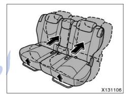
1. Hold the center of the lever and pull it up. Then slide the rear/second تلفن شبانه روزی: ۱-۸۸۸۶۲ ما seats fully backward and pull it forward slightly until it locks.
