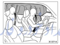
The SRS (Supplemental Restraint System) side airbags and curtain shield airbags are designed to provide further protection for the driver, front passenger and rear/second passengers in addition to the primary safety protection provided by the seat belts.
