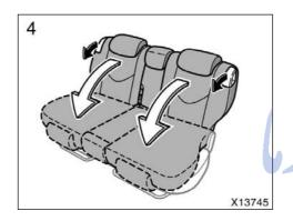
Pull down the seatback angle adjusting lever and fold down the seatback.
