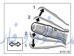
If the turn signal indicator lights (green lights) on the instrument panel flash faster than normal, a front or rear turn signal bulb is burned out. See "Replacing light bulbs" on page 422 in Section 7-3.
