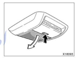
To open the display, push the lock release button.
