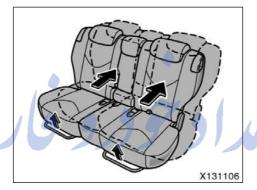
BEFORE USING LUGGAGE COVER Move the rear/second seats to the rear-شبانه روزی: ۵۰ most lock position.
