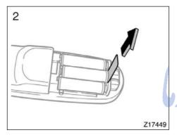
2. Remove the insulating sheet.
