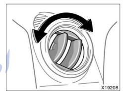
You can change air flow direction by turning the side vents.
