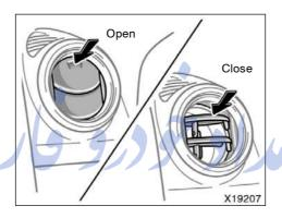
If air flow control is not satisfactory, check the side vents. The side vents may be incopened or closed as shown.
