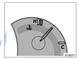
The gauge indicates the engine coolant temperature when the engine switch is in the "ON" position. The engine operating temperature will vary with changes in weather and engine load.
