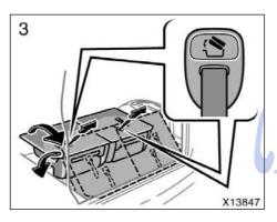
Pull and hold the seat lock release strap and lift up the seat rearward. Then push the seat down.
