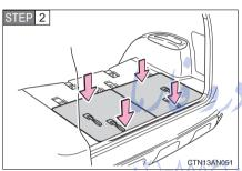
Push the seat on the front side against the floor and push the seat on rear side against the floor.
