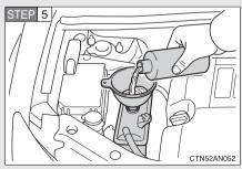
Add engine coolant if necessary.
