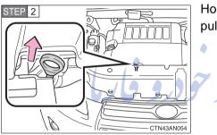
Hold a rag under the end and pull the dipstick out.
