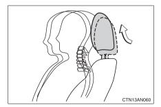
When the occupant's lower back presses against the seatback during a rear-end collision, the head restraint moves slightly forward and upward to help reduce the risk of whiplash on the seat occupant.
