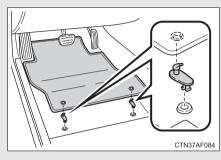
Fix the floor mat in place using the retaining hooks (clips) provided.
