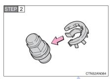
Vehicles with aluminum wheels and a steel wheel for the spare: Remove the plastic rings from the wheel nuts of the spare tire carrier.
