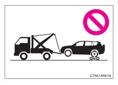
Do not tow with a sling-type truck to prevent body damage.
