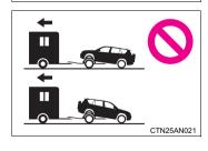
4WD models: Never tow this vehicle with any of the wheels on the ground. This may cause serious damage to the transmission and active torque control 4WD system.
