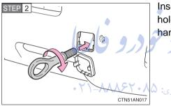
Insert the towing eyelet into the hole and tighten partially by hand.
