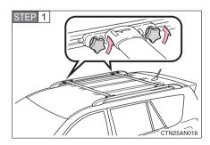
Turn the knobs counterclockwise to release the cross rails.
