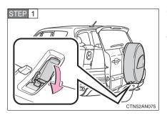
Open the back door. Unlock the latch handle which is on the bottom of the spare tire cover.
