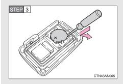
Remove the depleted battery.
