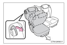
Pull the lever forward and fold down the seatback. The seat will slide forward.
