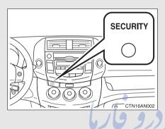
Vehicles without smart key system: The indicator light flashes after the key has been removed from the engine switch to indicate that the system is operating.
