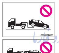
2WD models: Never tow this vehicle from the rear with the front wheels on the ground. This may cause serious damage to the transmission. If towing from the rear, used towing dolly.
