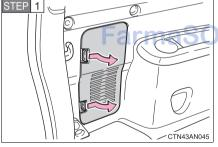
Open the back door ( $\rightarrow$ P. 46) and remove the cover.
