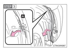
Move section "A" of the fender liner to the inner side of the vehicle, partly removing it and thereby allowing access to the front fog light.
