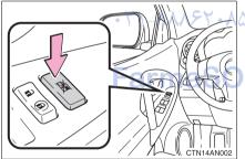
Press the switch down to lock the passenger window switches.
