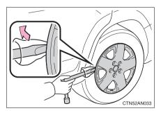
To protect the wheel ornament, place a rag between the wrench and the wheel ornament, as shown in the illustration. ▶ 17-inch and 18-inch wheels
