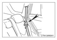
Pass the outer seat belts through the seat belt hangers and secure the seat belt plates to prevent the shoulder belts from being damaged.
