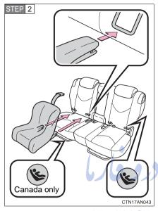
Latch the buckles onto the LATCH anchors.
