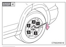
Firmly tighten each nut two or three times in the order shown in the illustration.
