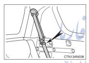
Pass the seat belts through the seat belt hangers to prevent the shoulder belts from being damaged.
