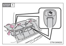
Pull and hold the seat lock release strap and lift up the seat rearward and then push the seat down.
