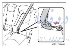
Second center seat: Release the center seat belt as shown in the illustration after removing the child restraint.
