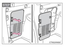
Disengage the claws and remove the cover.
