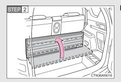
Fold up the deck board. The lid can be removed.
