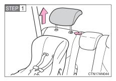
Remove the head restraint.
