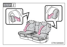
Pull down the seatback angle adjustment lever and fold down the seatback.
