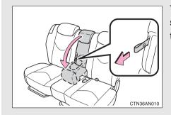
To use the armrest, pull the strap forward and fold down the center seatback.
