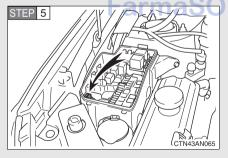
Remove the fuse with the pullout tool.
