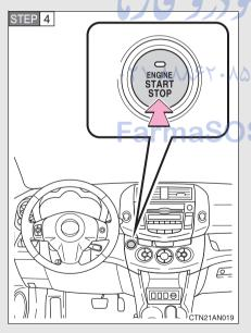
Press the "ENGINE START STOP" switch.
