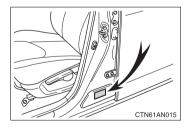
For the GAWR, see the Certification Label. For the maximum load of the tire, see the load limit at maximum cold tire inflation pressure mentioned on the sidewall of the tire. ( $\rightarrow$ P. 477)
