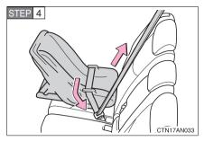
While pushing the child seat down into the rear seat, allow the shoulder belt to retract until the child seat is securely in place.
