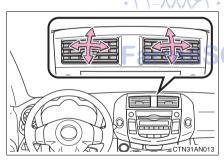
کفن شیانه روزی: Direct air flow to the left or right, up or down. ► Front outlets (right and left sides)
