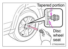
Tighten the nuts until the tapered portion comes into loose contact with the disc wheel seat. ▶ Replacing an aluminum wheel with an aluminum wheel
