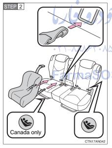
Fold the seatback while pulling the lever. Return the seatback and secure it at the 1st lock position (most upright position). Adjust the seatback to the 3rd lock position. ( $\rightarrow$ P. 54)
