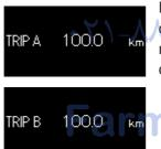
Displays the distance the vehicle has been driven since the meter was last reset. Trip meters "A" and "B" can be used to record and display different distances independently.
