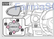
To adjust the mirror, press the switch.
