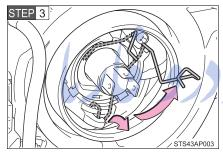
Release the bulb retaining spring.
