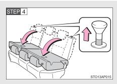
Pull the seatback lock release knob and fold the seatback down.
