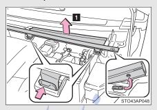
1 Pull the rubber strip on the edge to unhook it from the cover, and then push the tabs in and lift the cover off.
