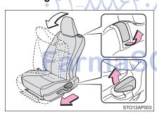
Lift the seatback lock release lever or seatback angle adjustment lever.
