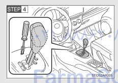
Press the shift lock override button with a flathead screwdriver or equivalent.
