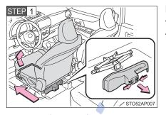
Move the front left seat to the front most position and remove the cover.
