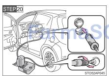
After driving for about 5 km (3 miles), stop your vehicle in a safe place on a hard, flat surface and remove the air release cap from the hose before reconnecting the repair kit.
