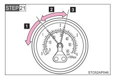
Turn the compressor switch on and wait for an approximately 5 seconds, and then turn it off. Check the tire inflation pressure.
