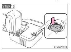
To inject the sealant and inflate the tire, turn the compressor switch on.
