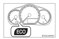
During Eco-friendly acceleration operation (Eco driving), Eco Driving Indicator Light will turn on. When the accelerator pedal is depressed excessively, and when the vehicle is stopped, the light turns off.
