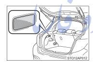
The luggage compartment light turns on when the back door is opened.
