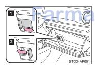
Air from the air conditioning system can be distributed into the glove box by opening and closing the vent.
