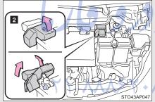
Remove the battery terminal cover and then the fuse box cover.
