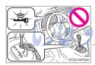
Vehicles with a Multidrive: Check that the shift lever is securely set in P. The engine may not start if the shift lever is displaced out of P. The smart entry & start system indicator light (green) will flash quickly.
