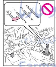
Do not shift the shift lever to R without depressing the clutch pedal.
