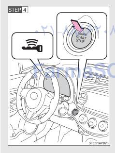
Press the "ENGINE START STOP" switch.
