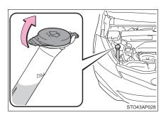
If the washer fluid level is less than "FULL" line, add washer fluid to "FULL" line.
