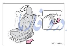
Lift the seatback lock release lever.
