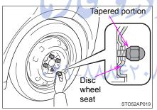
When replacing a steel wheel with a steel wheel (including a compact spare tire), tighten the wheel nuts until the tapered portion comes into loose contact with the disc wheel seat.
