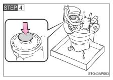
Operate the priming pump until fuel begins to run out.
