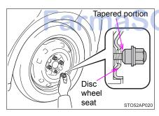
When replacing an aluminum wheel with a compact spare tire, tighten the wheel nuts until the tapered portion comes into loose contact with the disc wheel seat.
