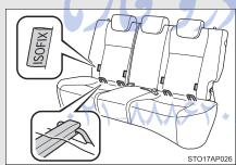
Vehicles with rear seats: ISO-FIX rigid anchors (ISOFIX child restraint system)
