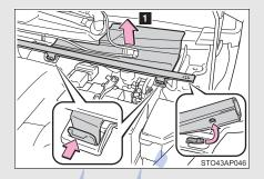
1 Pull the rubber strip on the edge to unhook it from the cover, and then push the tabs in and lift the cover off.
