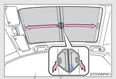
Pushing the tabs will release the lock, and the shade can be opened.
