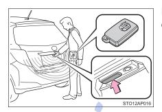
Press the button to unlock the door.
