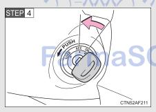
Vehicles without a smart entry & start system: Stop the engine by turning the engine switch to the "ACC" position.
