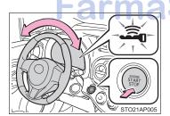
The smart entry & start system indicator light (green) will flash quickly.
