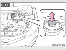
To bleed the fuel system, operate the priming pump until you feel more resistance.
