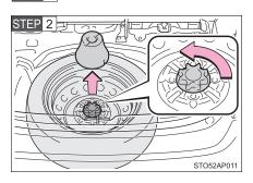
Remove the spare wheel cushion, then loosen the center fastener.
