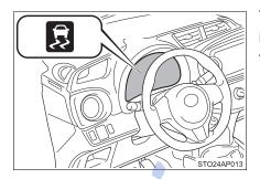
The slip indicator light flashes to indicate that the VSC/TRC systems have been engaged.
