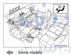
Air flows to the feet and the windshield defogger operates.
