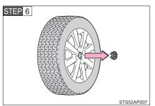
Vehicles with aluminum wheels: Remove the center wheel ornament by pushing from the reverse side.
