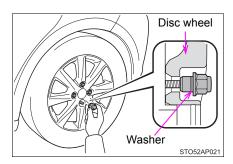
When replacing an aluminum wheel with an aluminum wheel, turn the wheel nuts until the washers come into contact with the disc wheel.
