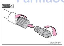
Attach the air release cap to the end of the hose.
