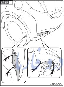
Remove the clips and remove the cover.
