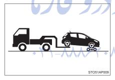
Vehicles with a Multidrive: Use a towing dolly under the front wheels.
