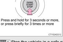
Vehicles with a smart entry & start system: To stop the engine, press and hold the STOP" "ENGINE START switch for 3 consecutive seconds or more, or press it briefly for 3 times or more in succession.
