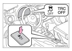
To turn the TRC and VSC systems off, press and hold the button for more than 3 seconds while the vehicle is stopped.
